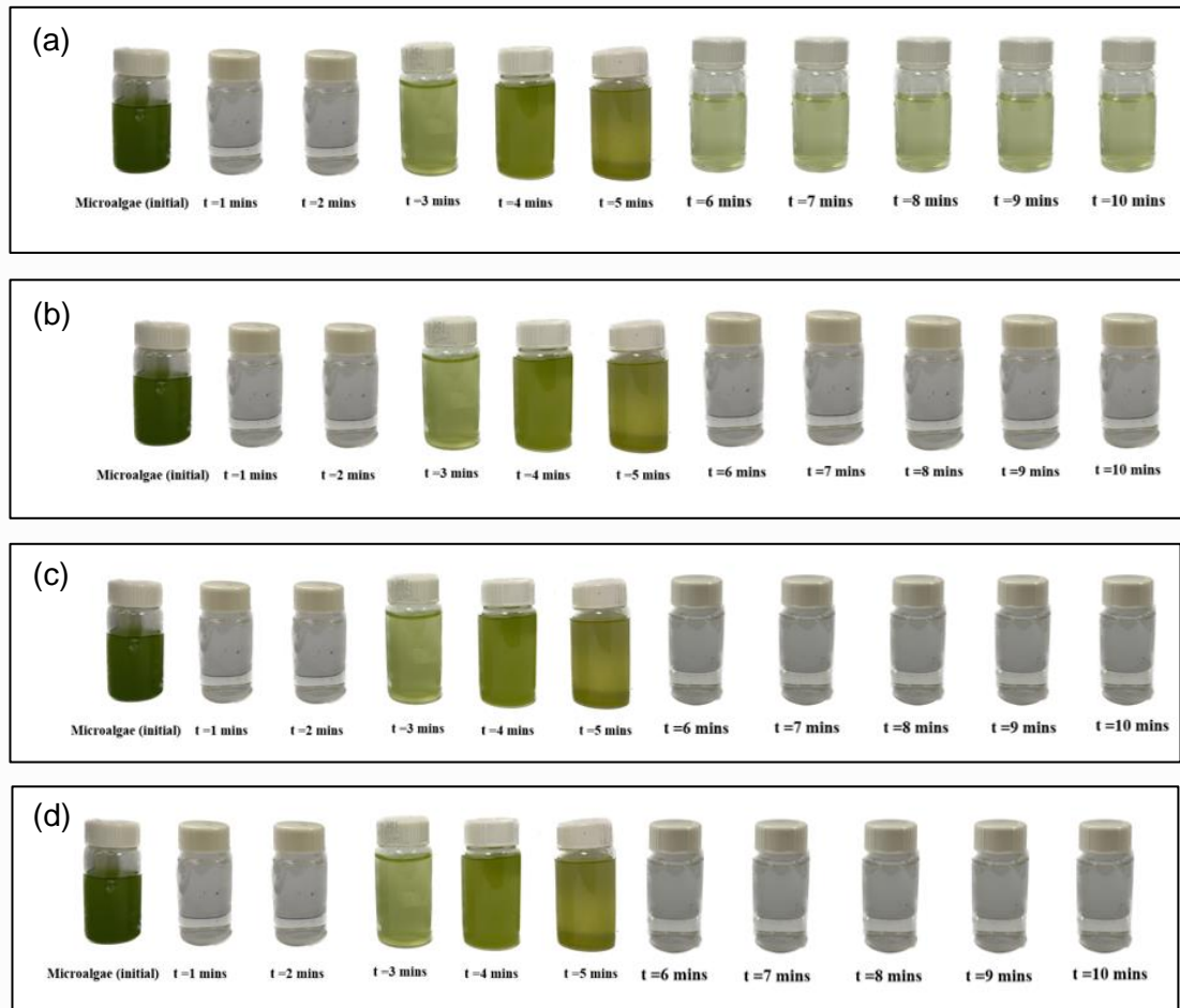
Figure 4.6: Photos of the collected effluent from the CF-LGMS-MH system at different time of the experiment, conducted under different baffle spacing for the static mixer: (a) no baffle; (b) 1.5D; (c) 2.0D; (d) 2.5D.
