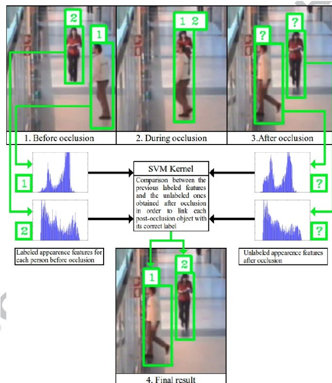
Figure 2.4 Graphical description of the proposed occlusion management method based on visual appearance. [8]
