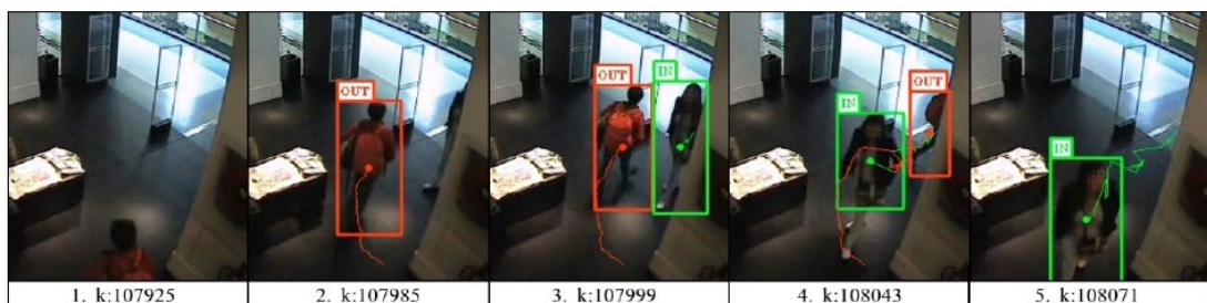
Figure 2.6 A real example of an alarm given off by detecting entry and exit events. [8]
