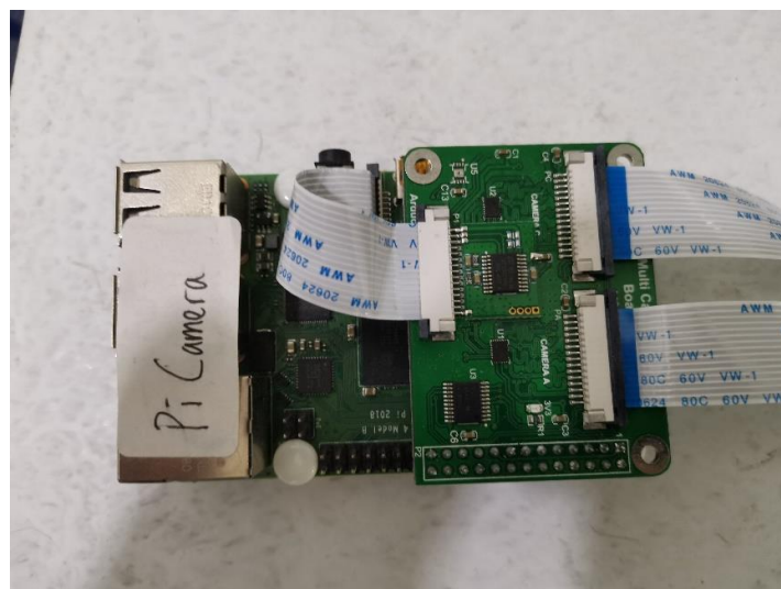
Figure 4.9: Integrated pi control board
