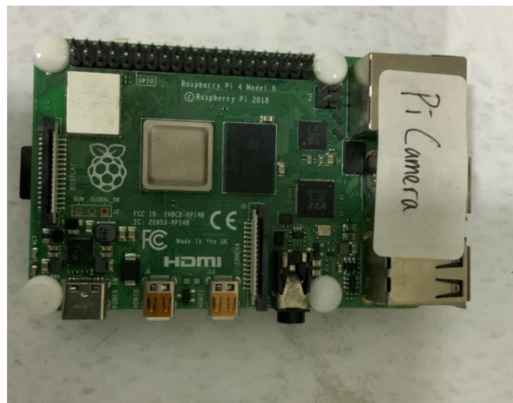
Figure 4.7: Control board of raspberry pi camera.
