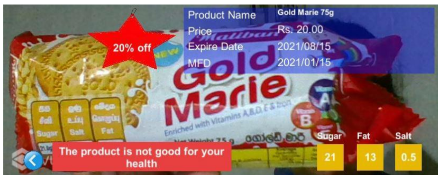
Figure 2.2: The user interface of the SAR application, displaying the warning messages
