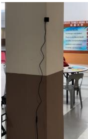
Figure 3.3: Setup of UP AI Edge – Full HD Machine Vision USB 2.0 Camera.
