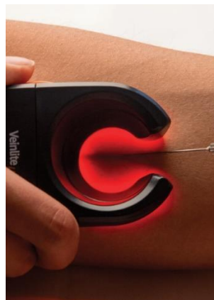
Figure 1.1: Transillumination Device from Veinlite (Veinlite, 2022).
