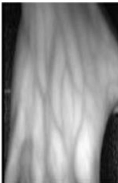
Figure 1.2: Dorsal Hand Vein Captured Using NIR Light Source (Sahana D S et al., 2020)
