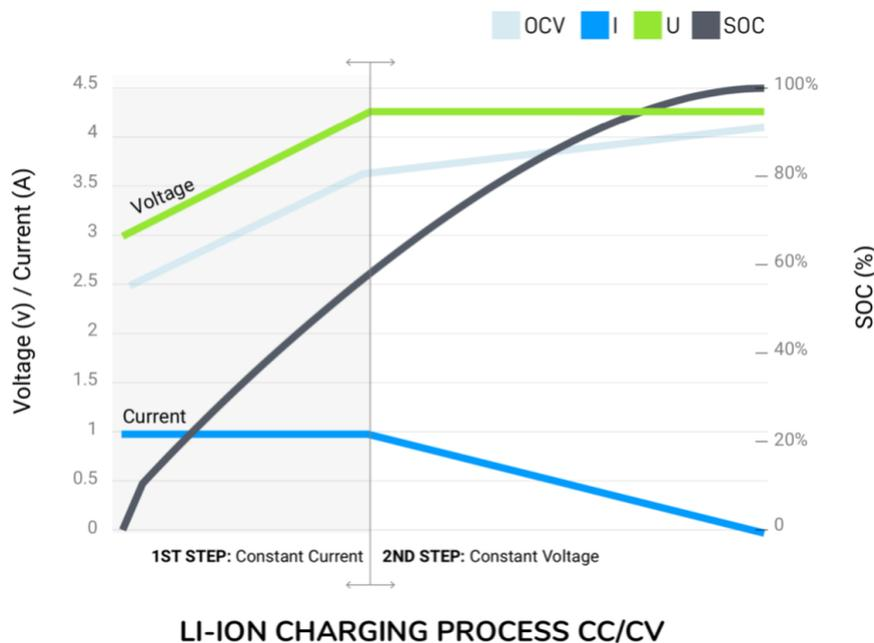
Figure 2.1: Ideal charging characteristics of Li-ion (Sourmey, 2022)
