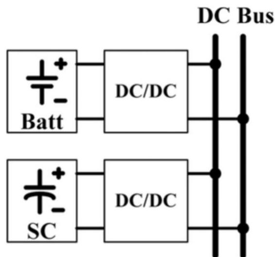
Figure 2.20: Parallel active HESS topology
