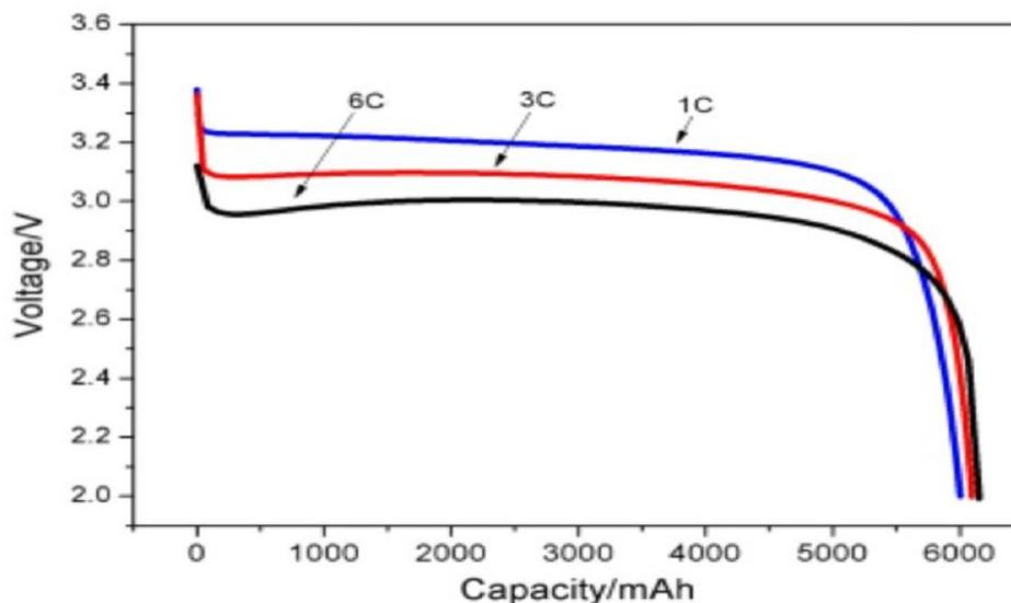
Figure 2.3: Discharge curve of lithium-ion battery at various C-rate
