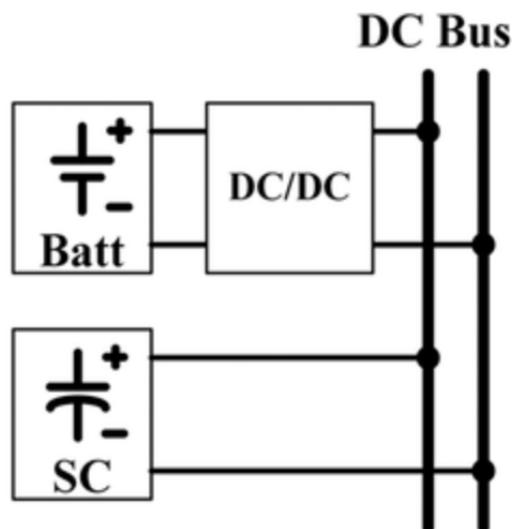
Figure 2.23: Battery semi-active HESS topology
