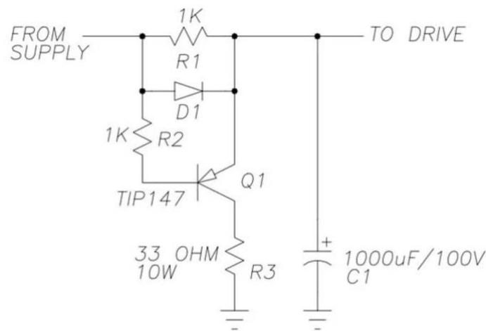
Figure 2.6: Dumping circuit
