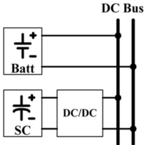
Figure 2.22: Supercapacitor semi-active HESS topology
