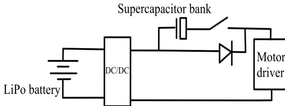
Figure 3.3: Draft of Proposed Power Conditioning Circuit for AGV
