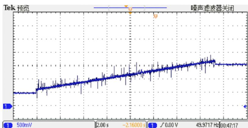
Figure 2.18: Waveform of electric brake energy recovery in supercapacitor bank (Cao, et al., 2019)
