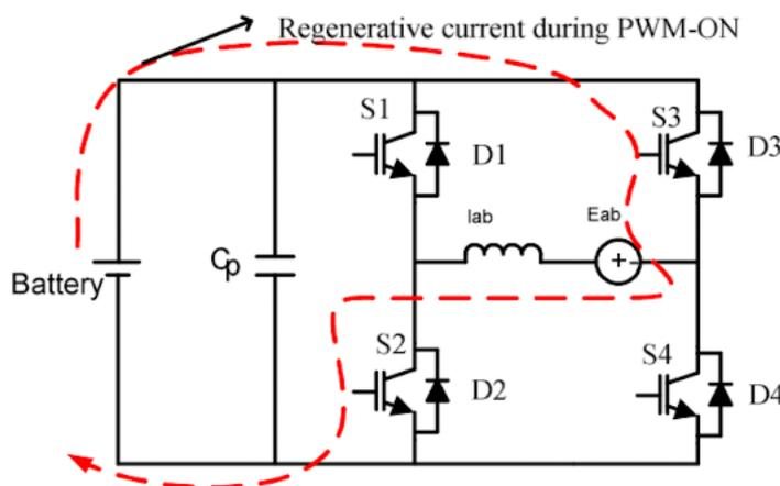
Figure 2.10: S2 and S3 closed with PWM-ON for regenerative. (Bobba & Rajagopal, 2010)
