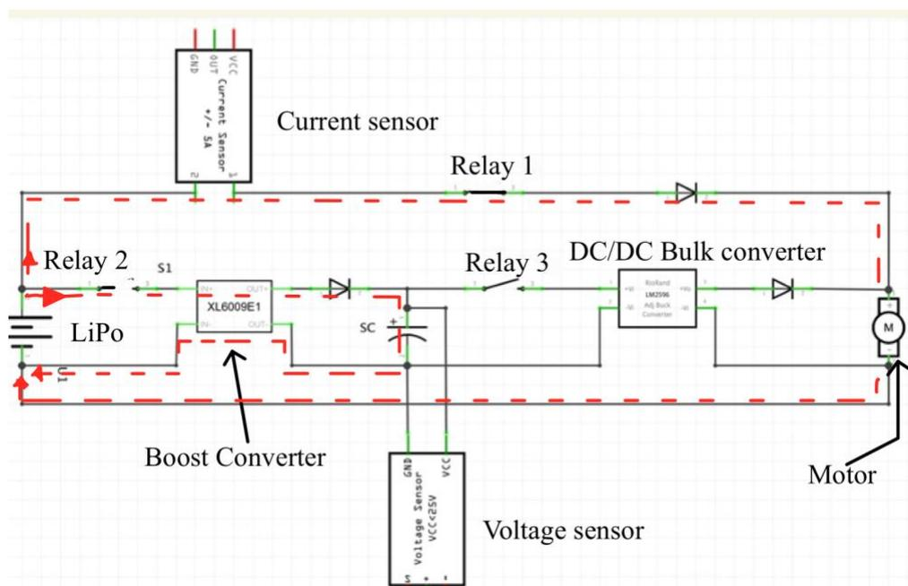
Figure 3.9: Current flow during charging supercapacitor and AGV moving.
