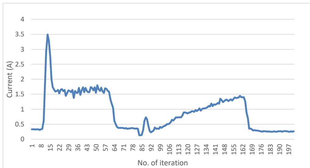
Figure 4.7: Effect of supercapacitor module to LiPo
