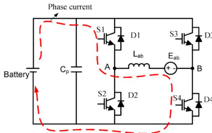
Figure 2.8: S1 and S4 are closed with PWM-ON for motoring. (Bobba & Rajagopal, 2010)
