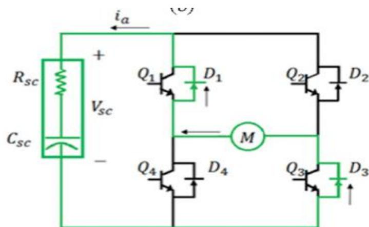
Figure 2.15: All switches closed during the charging of supercapacitor. (Adib & Dhaouadi, 2017)
