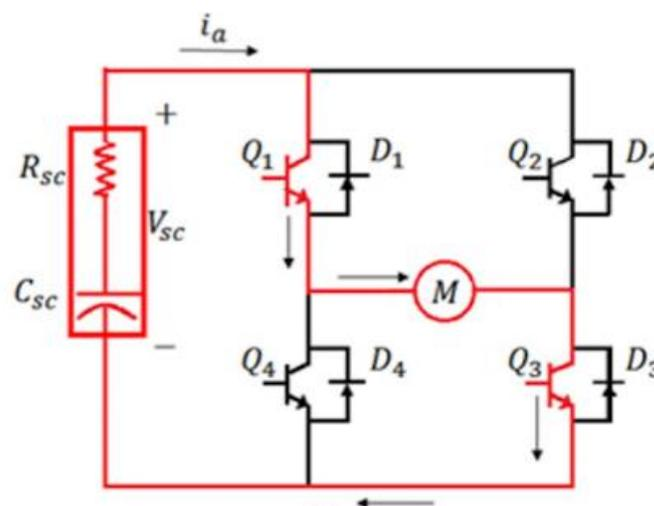
Figure 2.13: Q1 and Q3 closed for the motoring (Adib & Dhaouadi, 2017)
