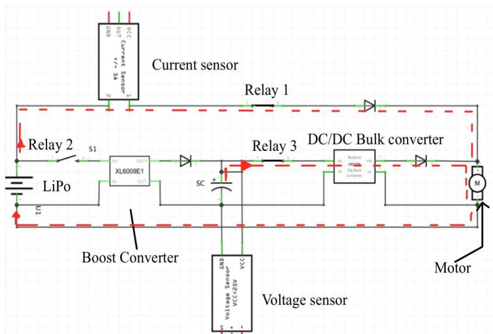
Figure 3.10: Current flow during supercapacitor kick in
