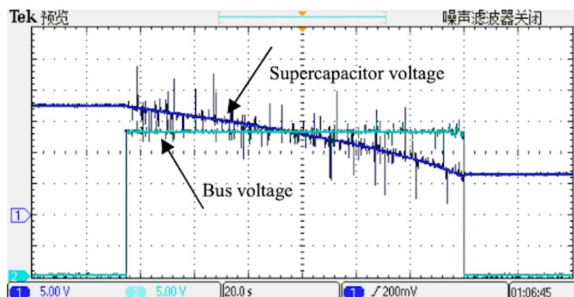
Figure 2.17: Waveform of bus voltage and supercapacitor voltage during motor starting state (Cao, et al., 2019)
