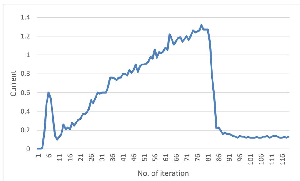
Figure 4.4: Current drawn out from LiPo with higher torque DC motors.
