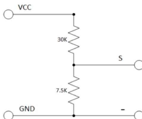
Figure 3.5: Schematic diagram of voltage divider in voltage sensor
