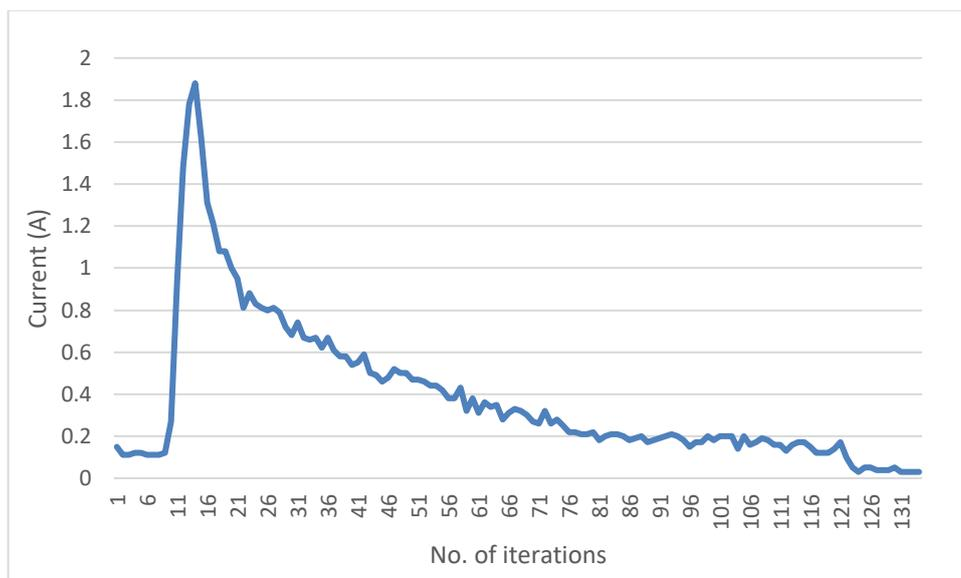
Figure 4.6: Current discharge of supercapacitor
