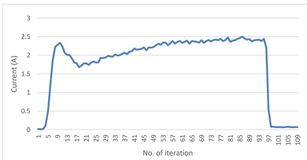
Figure 4.3: Current drawn out from LiPo with higher torque DC motors with supercapacitor connected.
