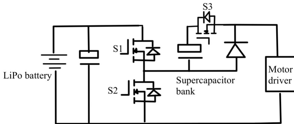
Figure 3.4: Schematic Diagram of Proposed Power Conditioning Circuit for AGV
