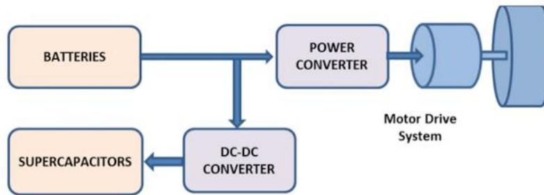
Figure 2.12: Topology of the battery-supercapacitor energy storage system (Adib & Dhaouadi, 2017)
