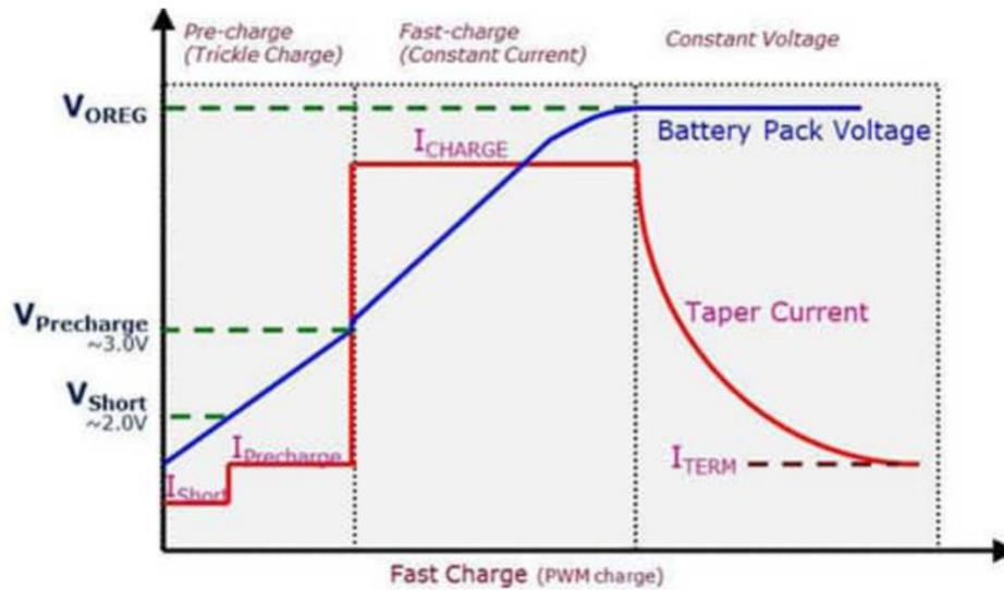
Figure 2.2: Realistic charging scenario of lithium-ion battery (Staff, 2021)
