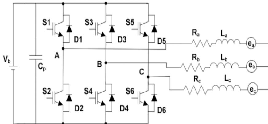
Figure 2.7: Proposed regenerative braking circuit (Bobba & Rajagopal, 2010)
