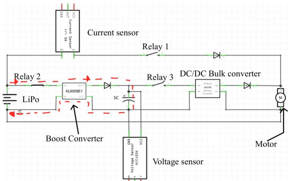
Figure 3.8: Current flow during charging of supercapacitor
