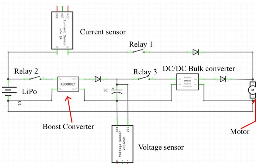
Figure 3.6: Schematic diagram of proposed circuit
