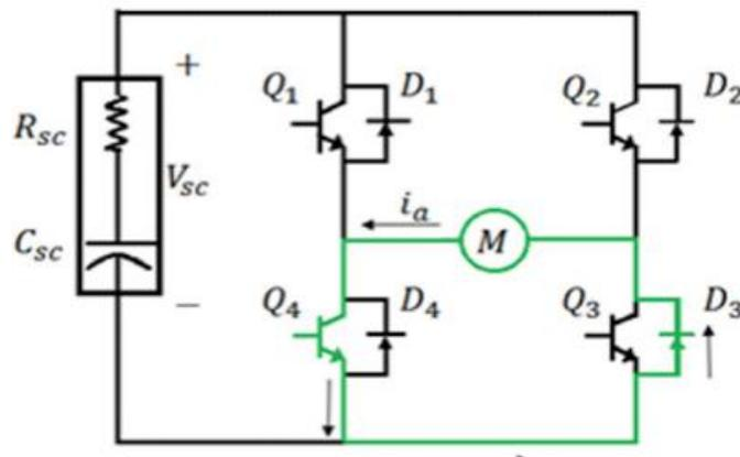
Figure 2.14: Q4 closed during freewheeling of motor. (Adib & Dhaouadi, 2017)
