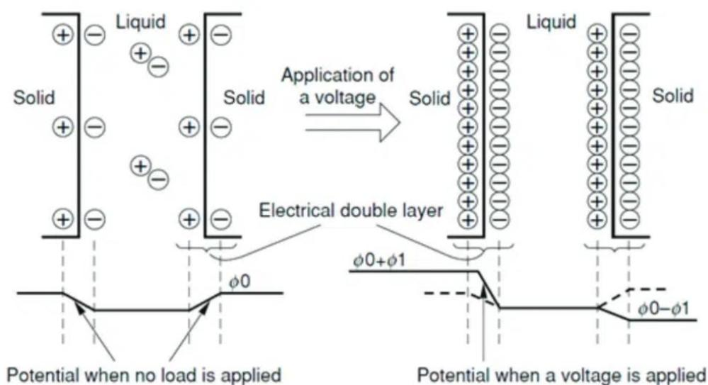
Figure 2.4: Basic structure of supercapacitor
