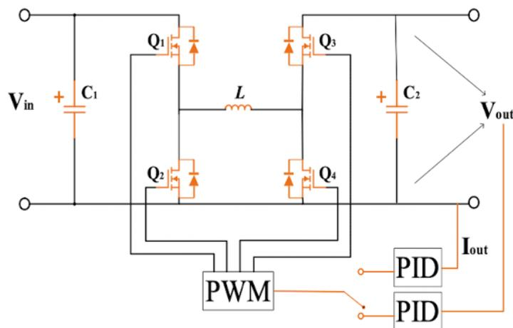
Figure 2.16: Topology of bidirectional synchronous rectification Buck-Boost circuit (Cao, et al., 2019)
