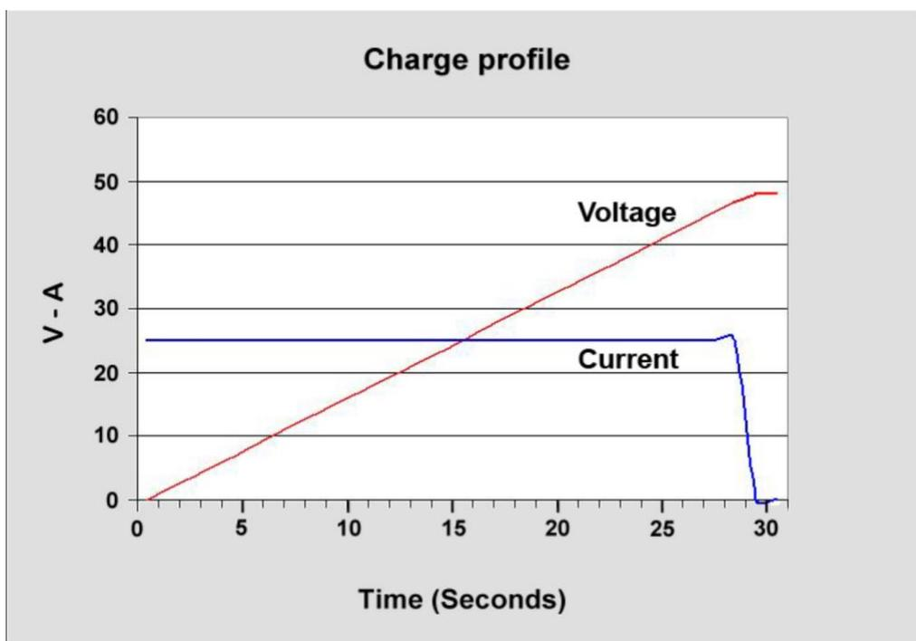
Figure 2.5: Charging profile of supercapacitor (Battery University,2021)
