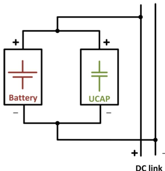
Figure 2.19:Passive HESS topology
