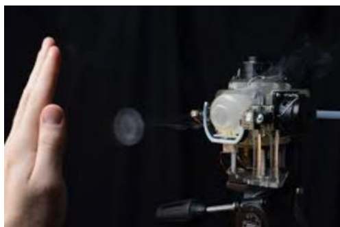
Figure 2.12: Illustration of Air Vortex Ring (Kirn, 2013)
