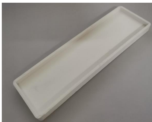
Figure 3.4: Molds created using Solidworks and 3D printed.
