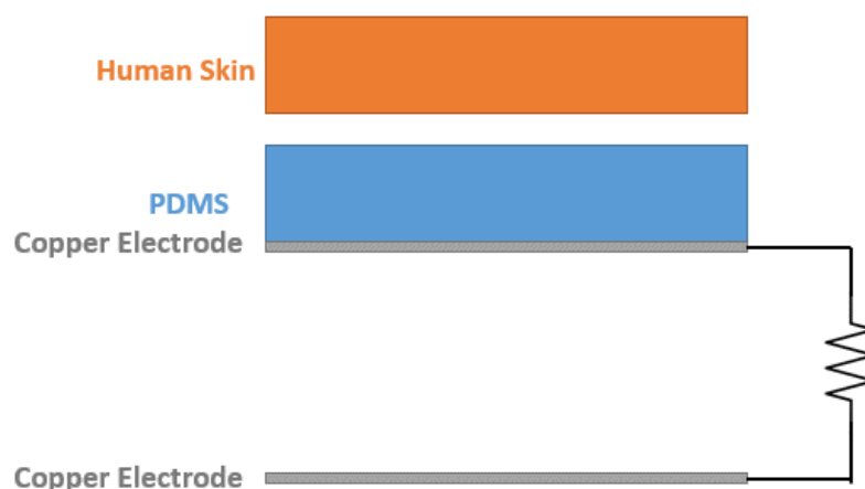
Figure 3.2: Schematic Diagram of Simulation Model for Single Electrode Mode.
