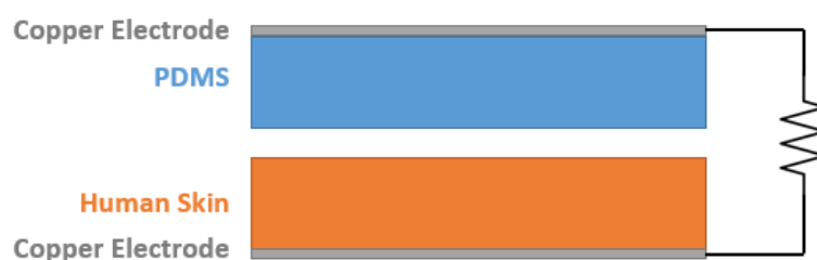
Figure 3.1: Schematic Diagram of Simulation Model for Contact Separation Mode.
