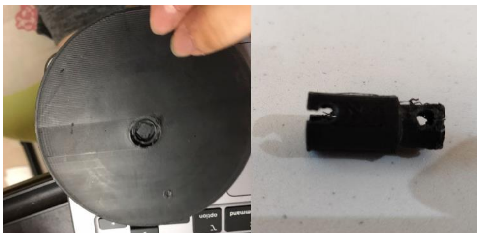
Figure 3.23 Broken driven pulley and coupler.
