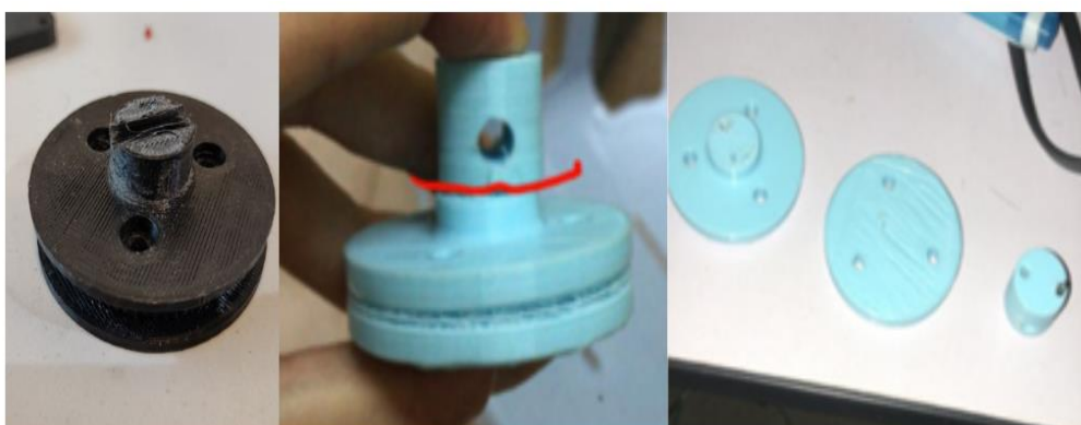
Figure 3.22 Broken reel coupler/driving pulleys.
