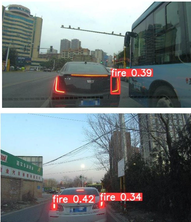
Figure 4.2: FP on car's back light in both YOLOv5s (Top) and Improved YOLOv5s (Bottom)
