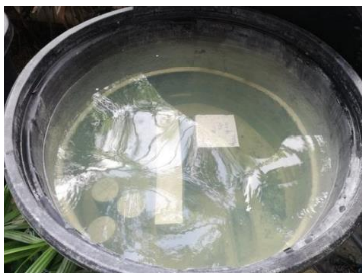
Figure 3.11: Concrete Samples Cured in Water.
