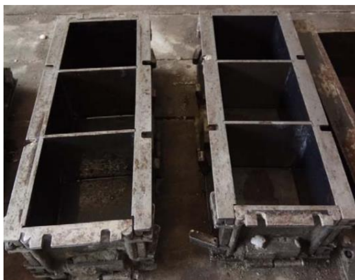
Figure 3.7: Cubical Steel Mould with 100 mm x 100 mm x 100 mm.
