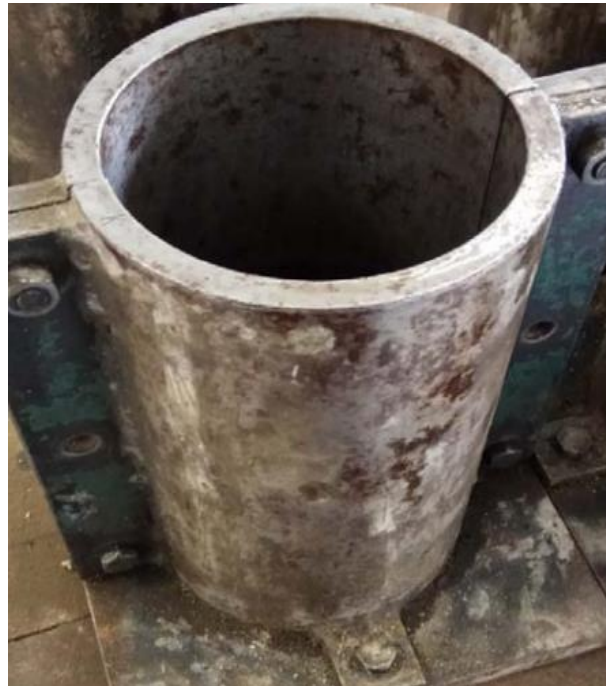
Figure 3.8: Cylindrical Steel Mould with 100 mm Diameter and 200 mm Height.
