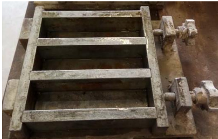
Figure 3.9: Prism Steel Mould with 40 mm Width x 40 mm Height x 160 mm Length.
