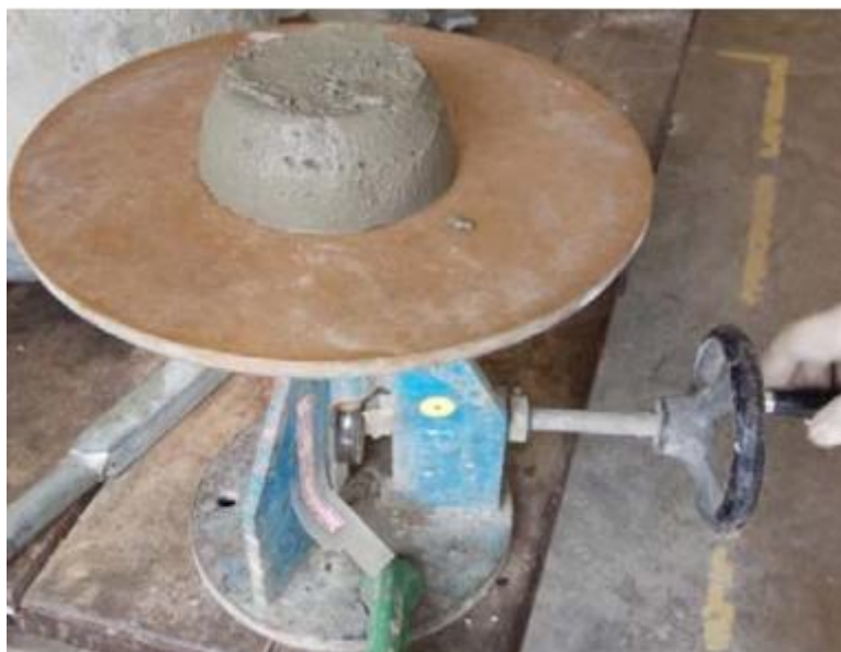
Figure 3.13: Flow Table Test.
