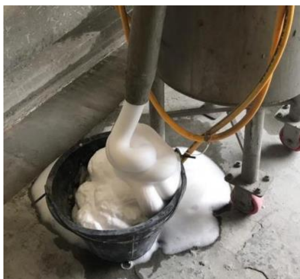
Figure 3.5: Foam Generated by Foam Generator.
