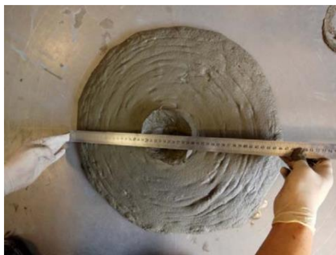
Figure 3.12: Measured Inner and Outer Diameter After Inverted Slump Test.
