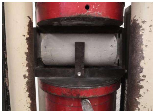
Figure 3.15: Splitting Tensile Strength Test with Cylinder Sample.
