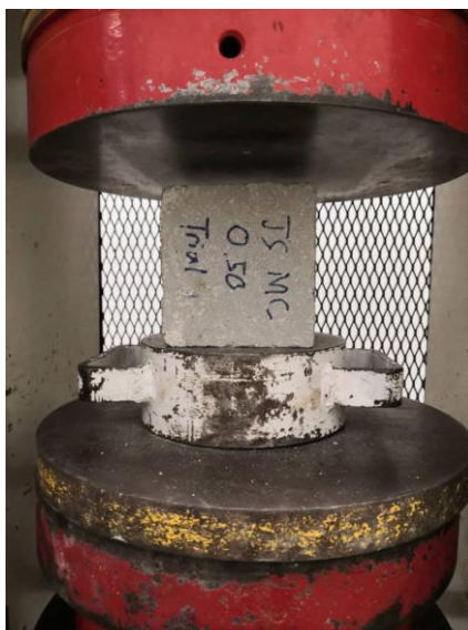
Figure 3.14: Compressive Strength Test with Cube Sample.
