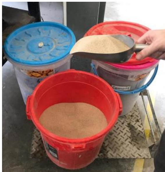
Figure 3.3: Fine Aggregate Sieved with 600 \mu\text{m} .
