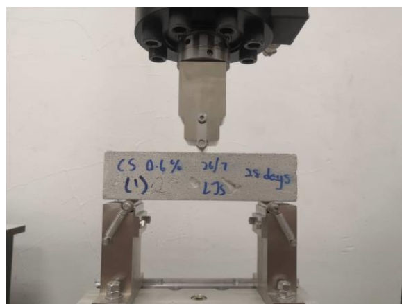
Figure 3.16: Flexural Strength Test with Prism Sample.
