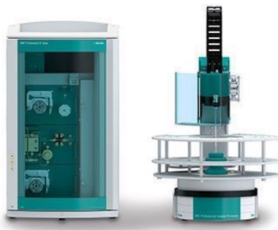
Figure 3.8: Ion chromatography (Metrohm, Metrosep Organic Acids-250/7.8)
