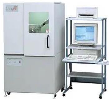
Figure 3.5: XRD (Shimadzu, XRD6000)
