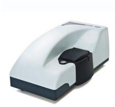
Figure 3.11: Zeta potentiometer (Malvern, Zetasizer Nano-ZS)
