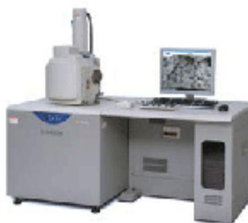
Figure 3.4: SEM-EDS (Hitachi, S-3400N)
