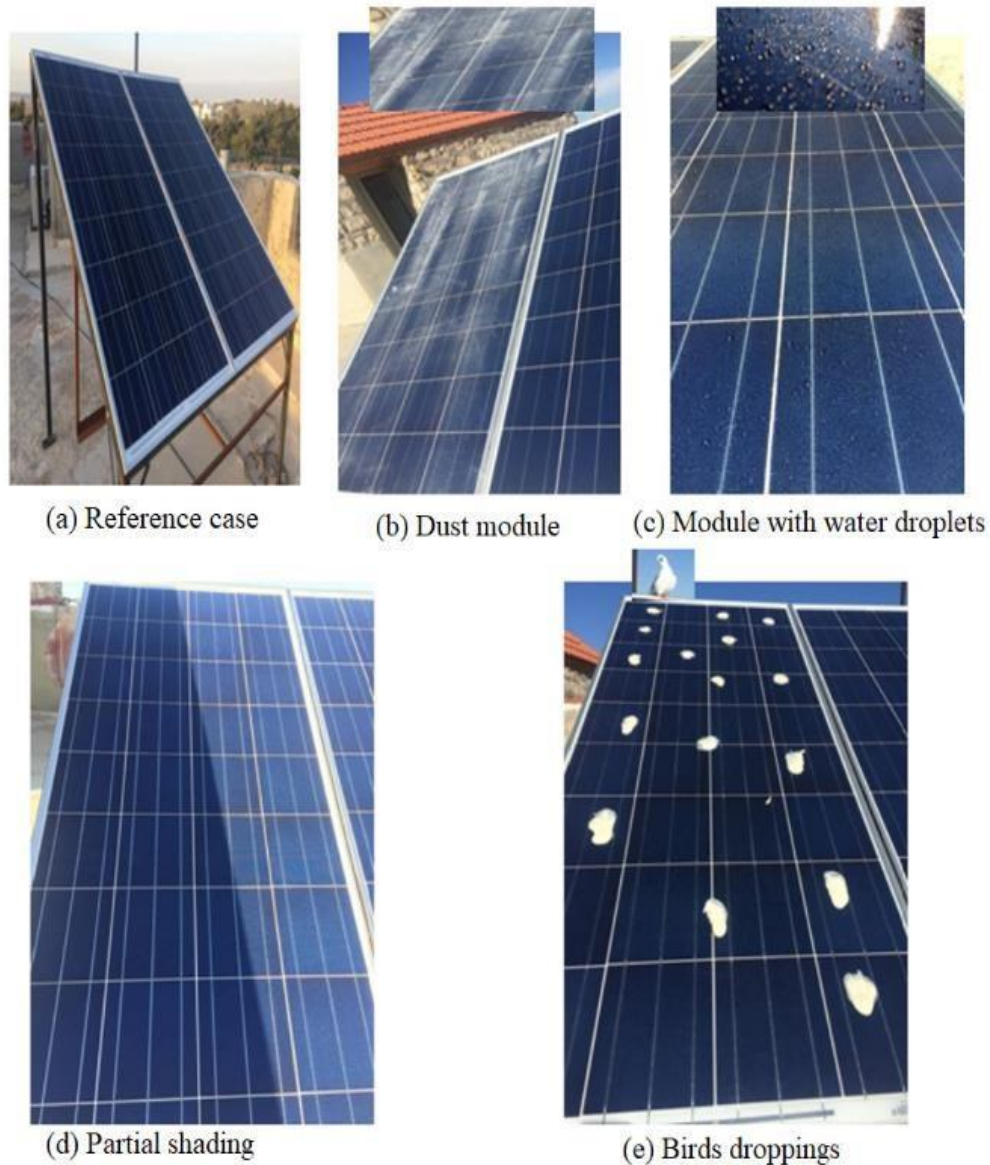
Figure 2.5: PV Panels in Different Conditions. (Mustafa et al., 2020)
