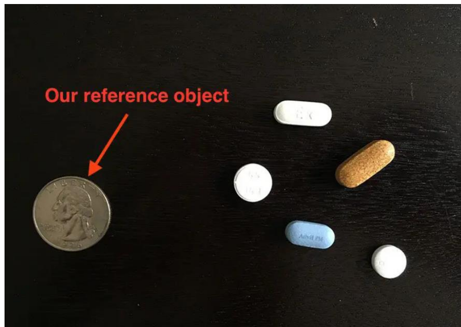
Figure 2. 11: Example of reference object placed in the image (Adrian,2021)
