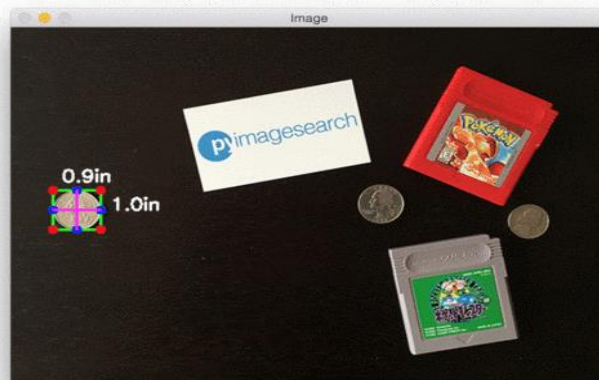
Figure 2. 12: Measuring object' size in an image with OpenCV and Python (Adrian,2021)
