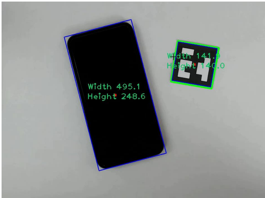
Figure 2. 16: Object's dimensions show with pixel
