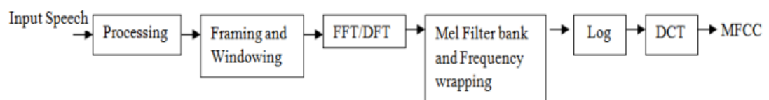
Figure 2.2: MFCC extraction schema (Srinivasan et al., 2014).
