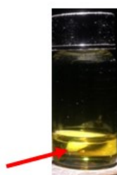
Figure 4.6: Suspension of White Floccule in the Perovskite Precursor Solution (Jia et al., 2017).
