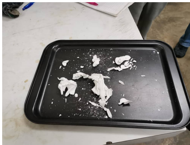
Figure B-2: Feedstock with 60 vol% Zirconia, binder ratio LDPE: PW, 40:60
