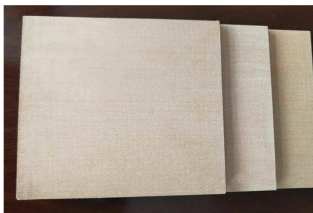
Figure 3.5: A Commercial MgO Board was used to Compare the Effectiveness of the Best-Performing Fire-Retardant Board.
