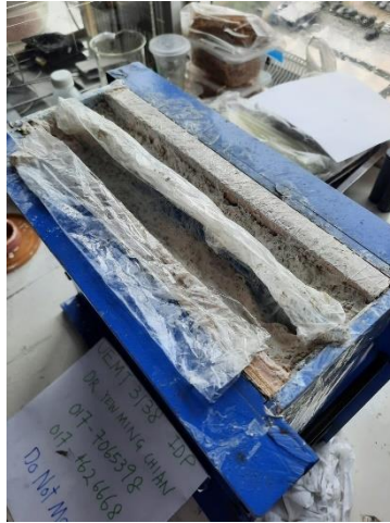
Figure 3.2: A Cast Iron Mould was used to Fabricate the Best-Performing Fire-Retardant Board core.
