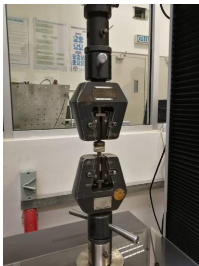
Figure 3.10: Experiment Setup for the Adhesion Strength Test.
