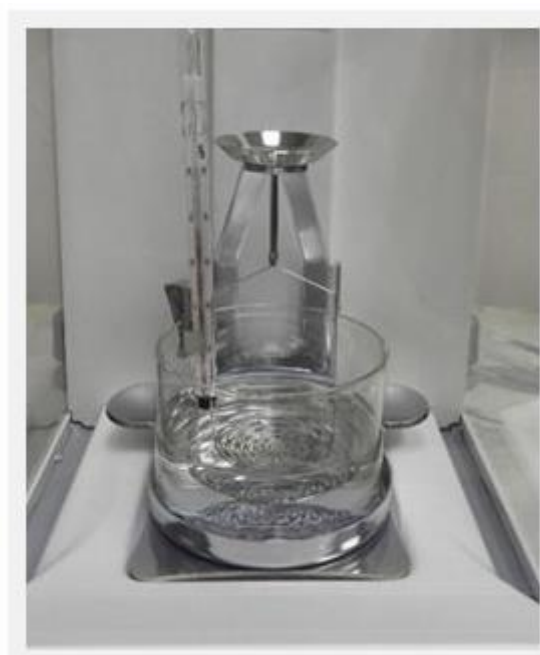
Figure 3.8: Diagram of the set up for water immersion density test (Anderson Materials Evaluation, Inc., n.d.).
