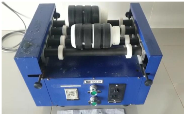
Figure 3.2: Ball milling for the alumina powder and \text{TiO}_2 powder.
