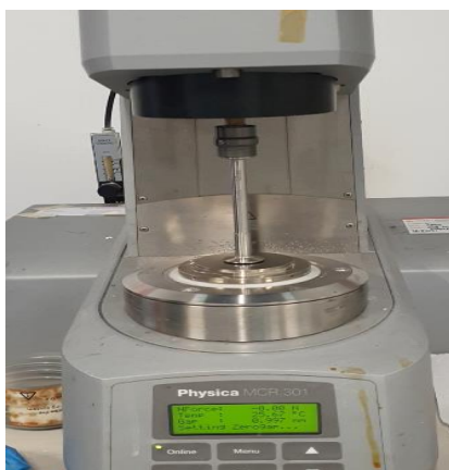
Figure 3.5: Diagram of rheometer with parallel plate system.
