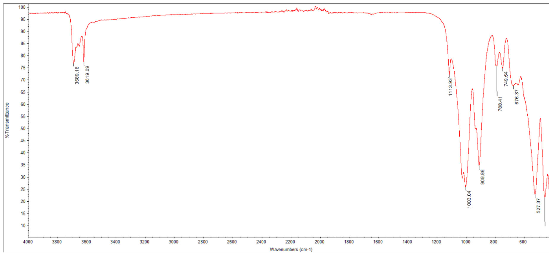
Figure 4.24: FTIR spectrum of Chinese kaolin treated with B. aryabhatai
