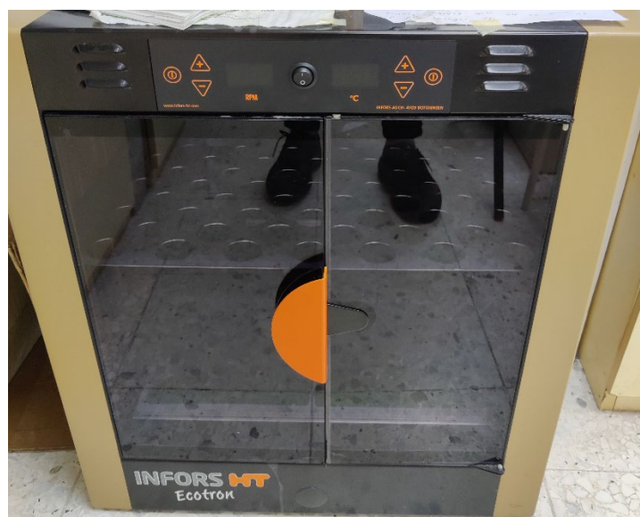
Picture B- 14: Incubator (INFORS HT Ecotron) to incubate Bacillus bacteria at 37 °C 250 rpm.
