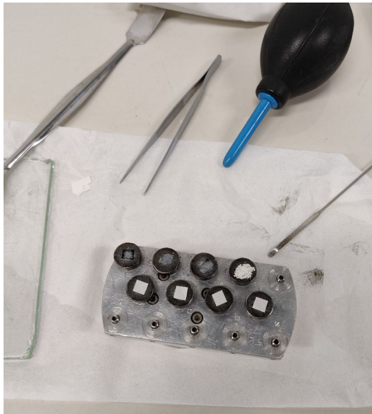
Picture B-21: Sample preparation for SEM-EDX.
