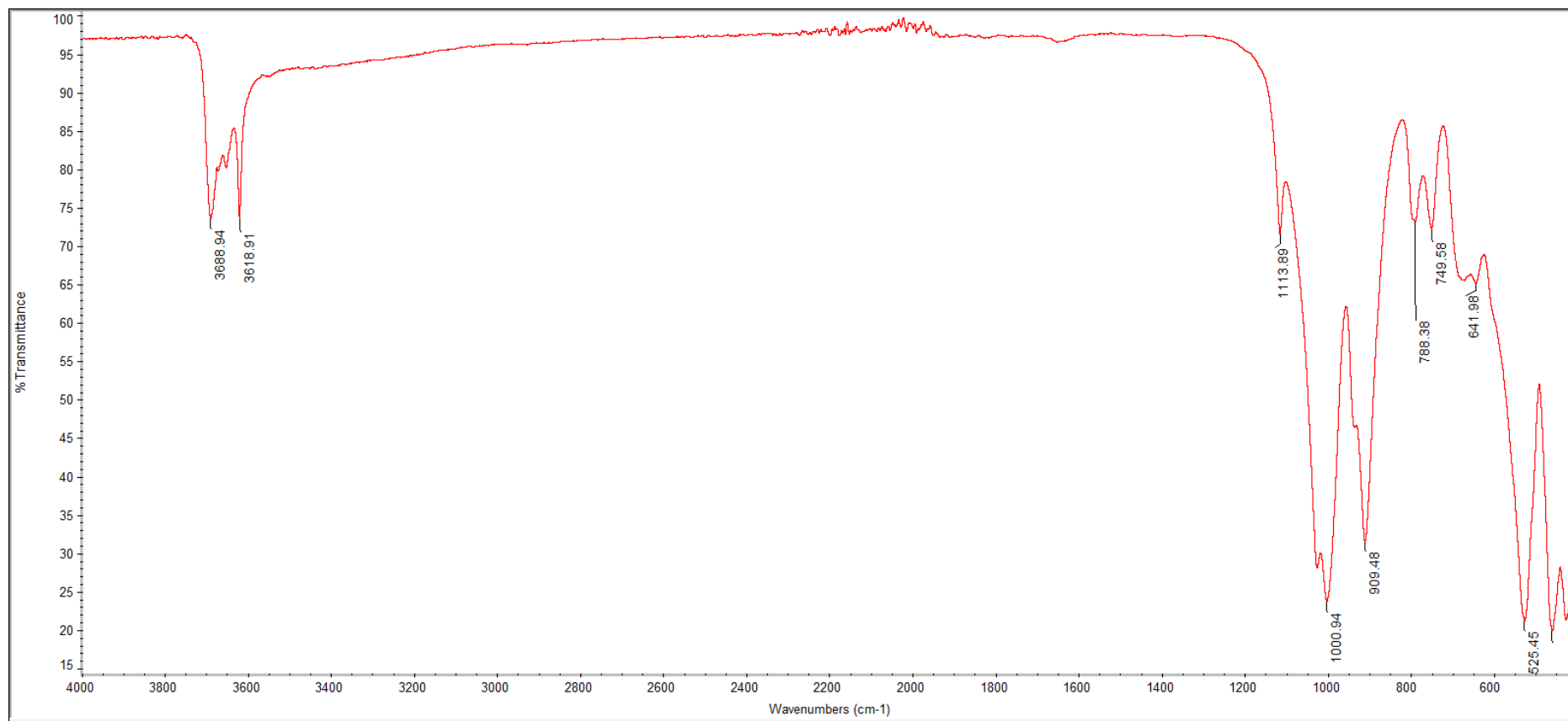
Figure 4.22: FTIR spectrum of Chinese kaolin treated with B. Cereus .
