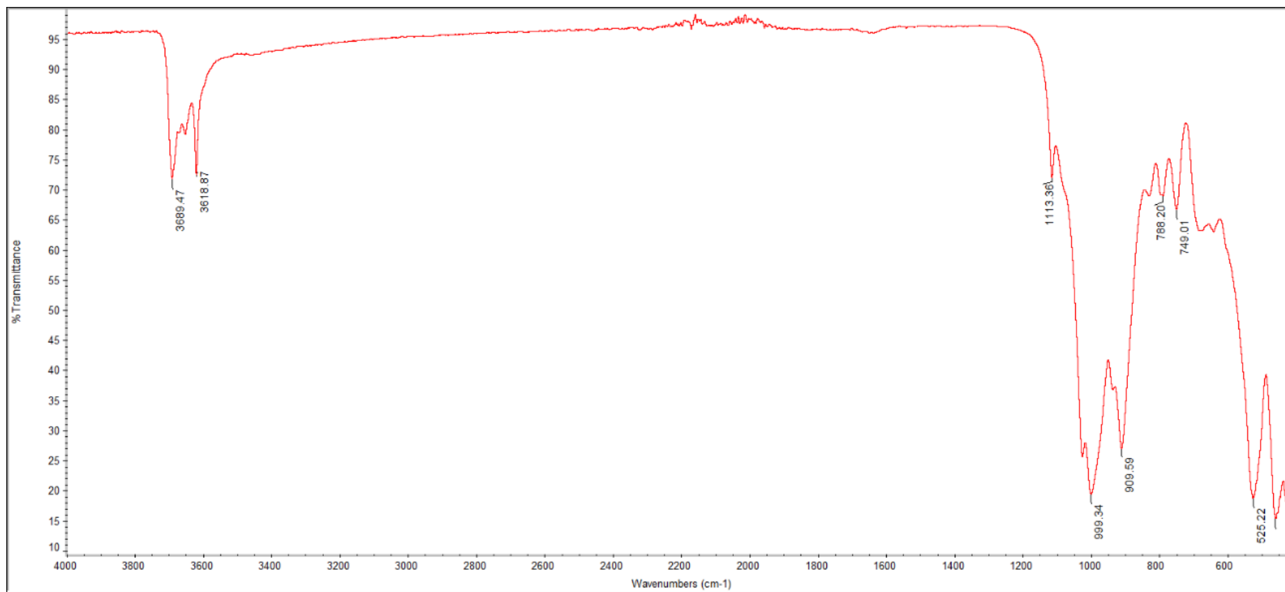
Figure 4.20: FTIR spectrum of Malaysian kaolin treated with B. megaterium .
