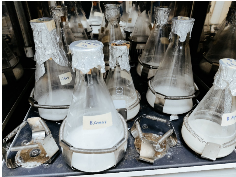
Picture B-13: Biobleaching of kaolin incubated at 30 °C 250 rpm.
