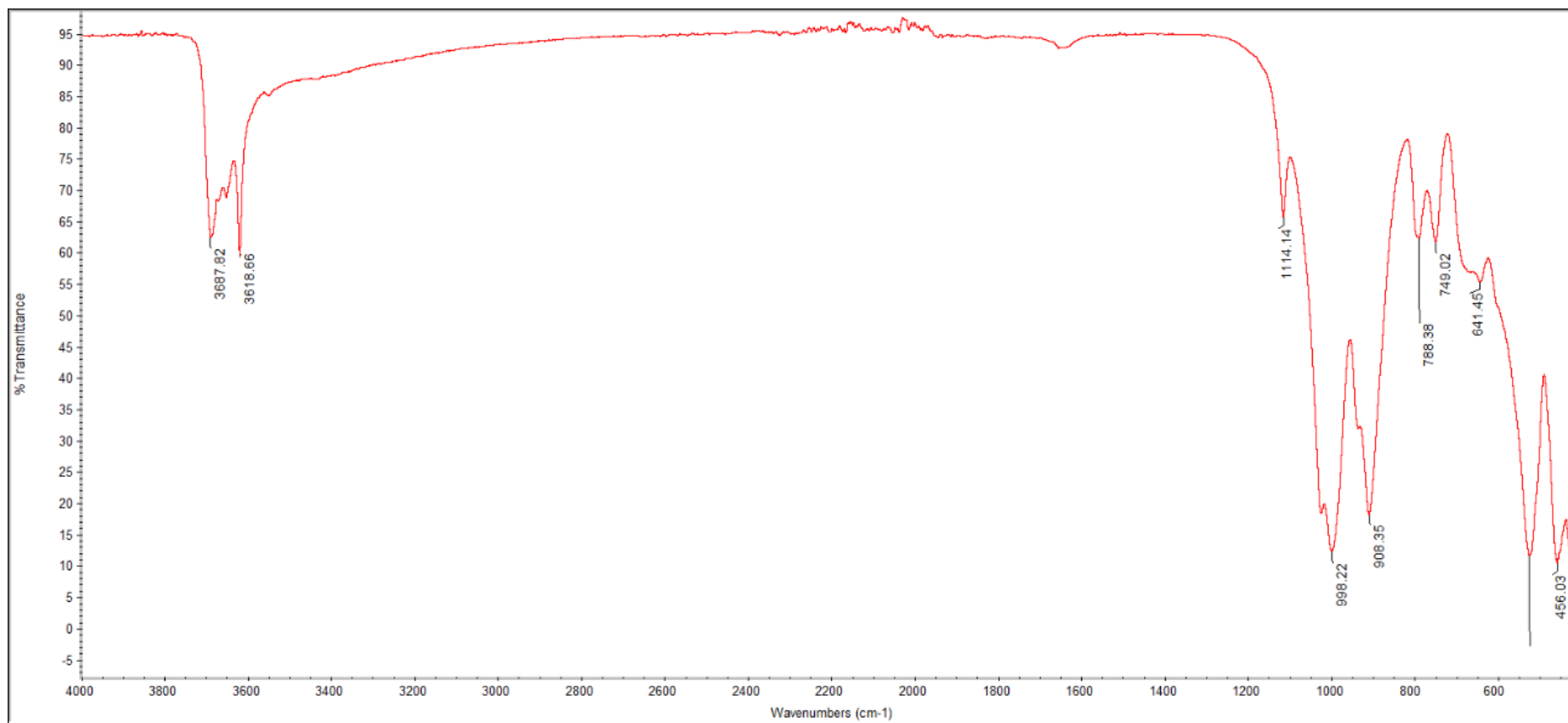
Figure 4.18: FTIR spectrum of raw Chinese kaolin.
