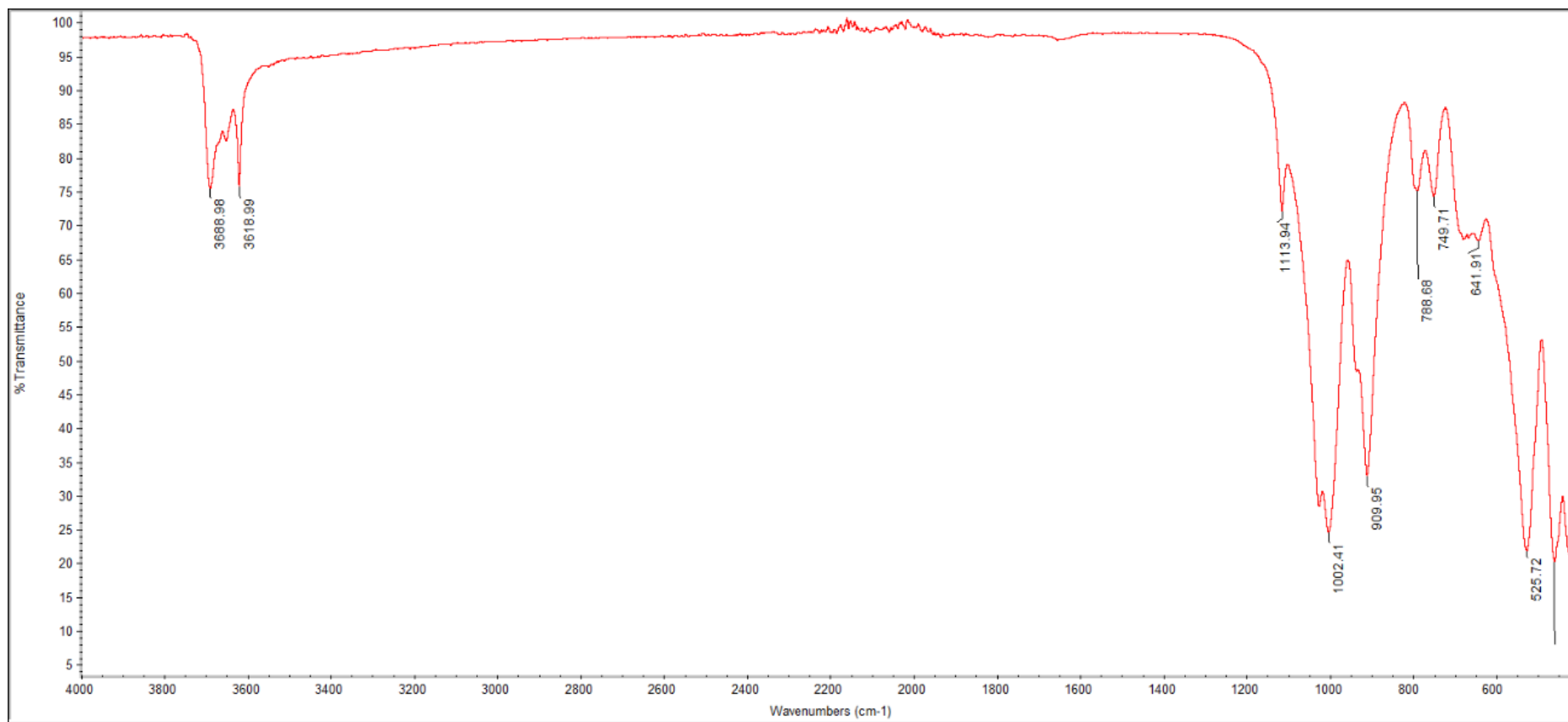
Figure 4.23: FTIR spectrum of Chinese kaolin treated with B. megaterium .
