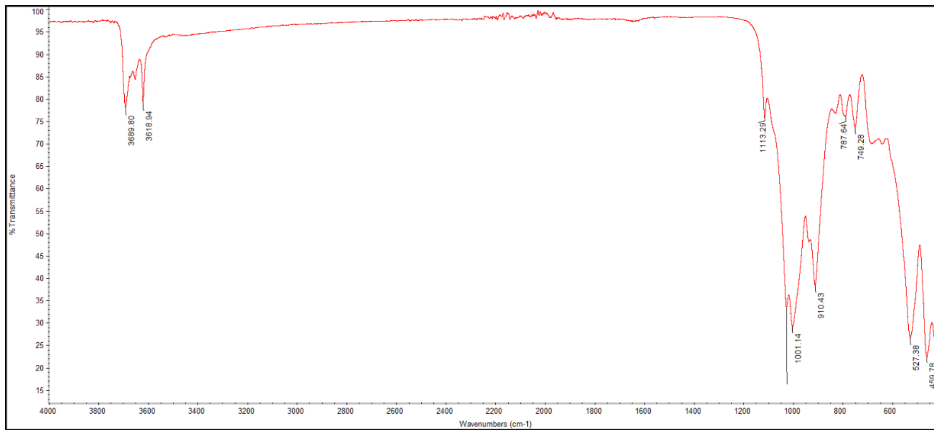
Figure 4.19: FTIR spectrum of Malaysian kaolin treated with B. cereus .
