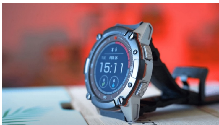
Figure 2.8: Matrix PowerWatch Powered by TEG and Body Heat (Tech4All, n.d.).
