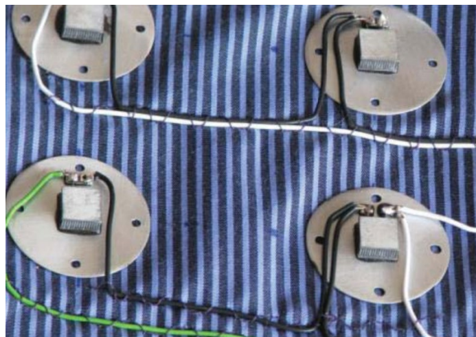
Figure 2.7: Electrocardiography (ECG) Shirt (Leonov, 2013).
