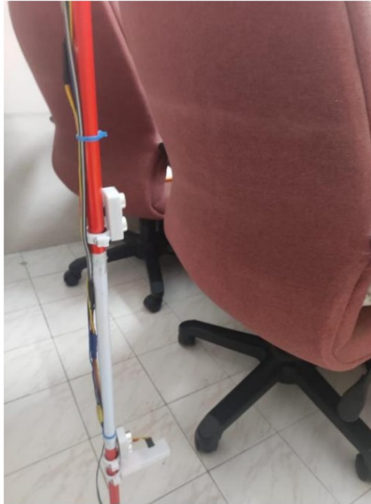
Figure B - 1: Technical Test for Obstacle Detection by Middle Sensor.
