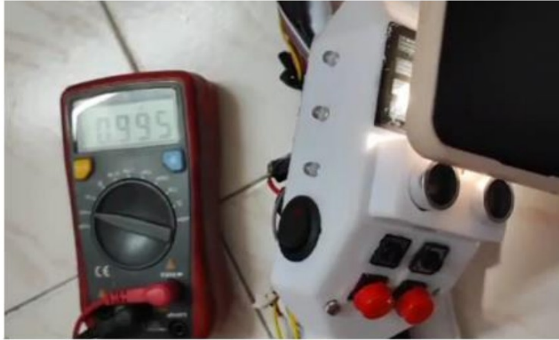
Figure 4.6: Testing of Voltage of Solar Panel.
