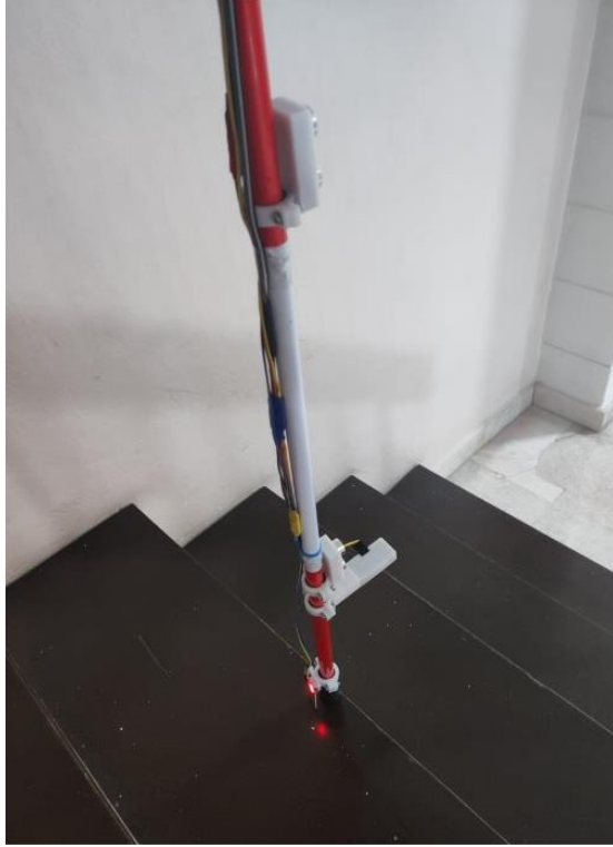
Figure B - 3: Technical Test for Staircase Detection Feature.
