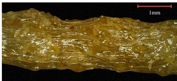
Figure 4.3: Section View of rPP/CHF with 7.5 wt% fiber content.
