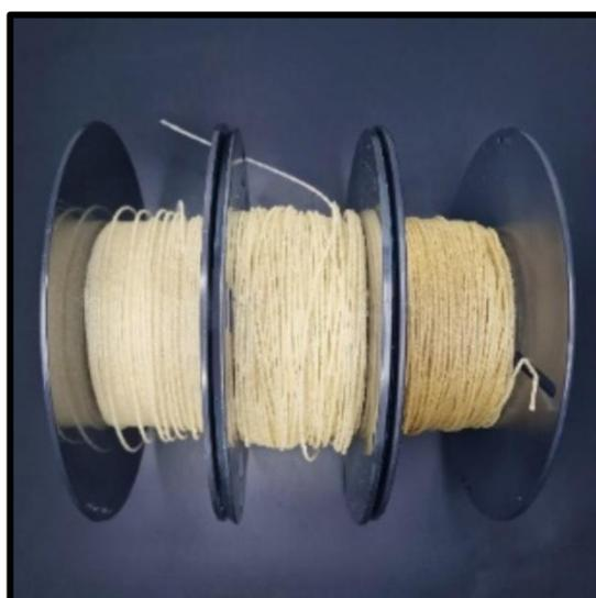
Figure 3.4: Extruded Composite Filaments from 2.5 wt% to 7.5 wt%.
