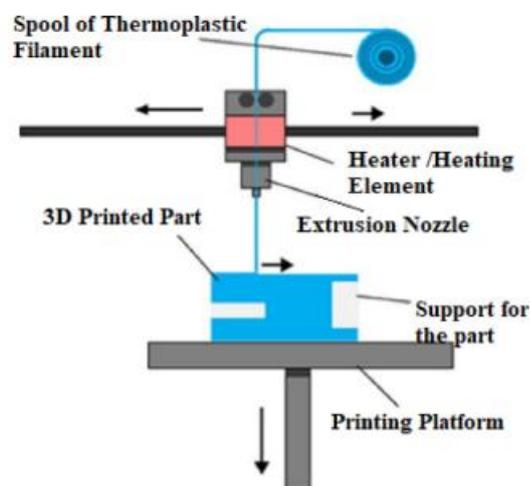
Figure 2.1: The Basic Components of an FDM 3D Printer (Jaisingh Sheoran and Kumar, 2020).
