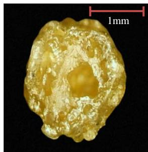
Figure 4.4: Cross-section of rPP/CHF with 7.5 wt% fiber content.
