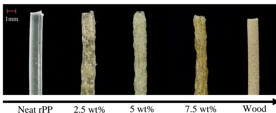
Figure 4.1: High Magnification View of the Filament Surface.
