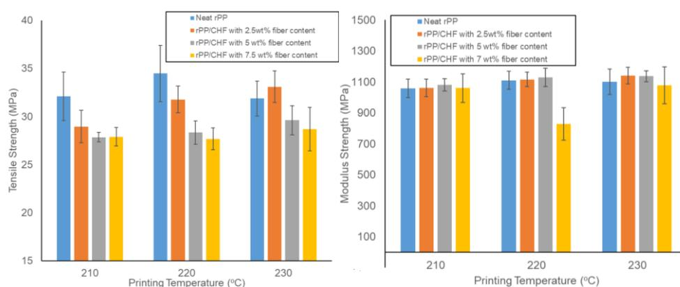
Figure 4.7: Result of Tensile and Modulus Strength.
