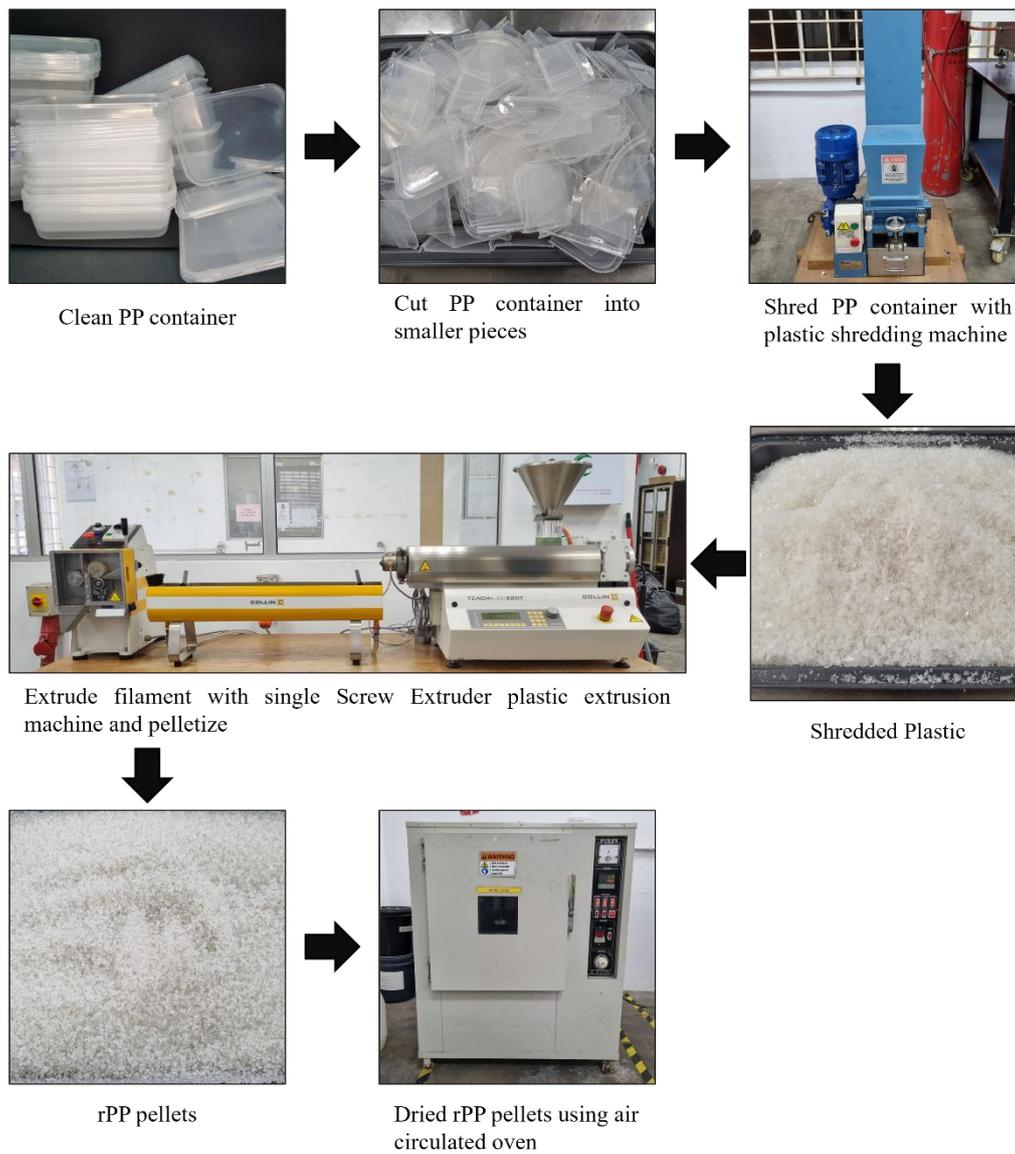
Figure 3.2: Process of Recycling PP Container into rPP Pellet.
