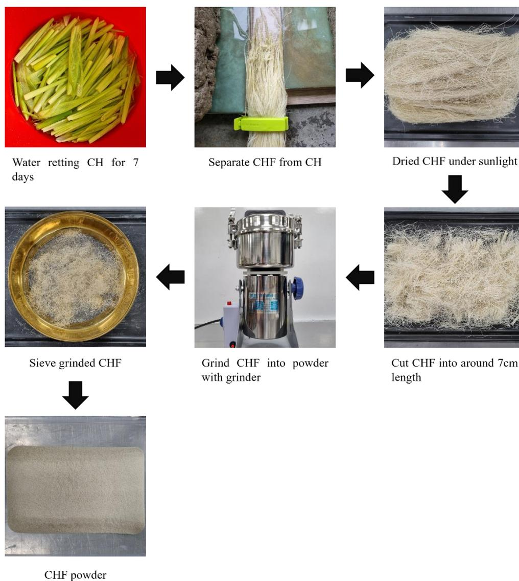
Figure 3.3: Process of Recycling CH into CHF Powder.
