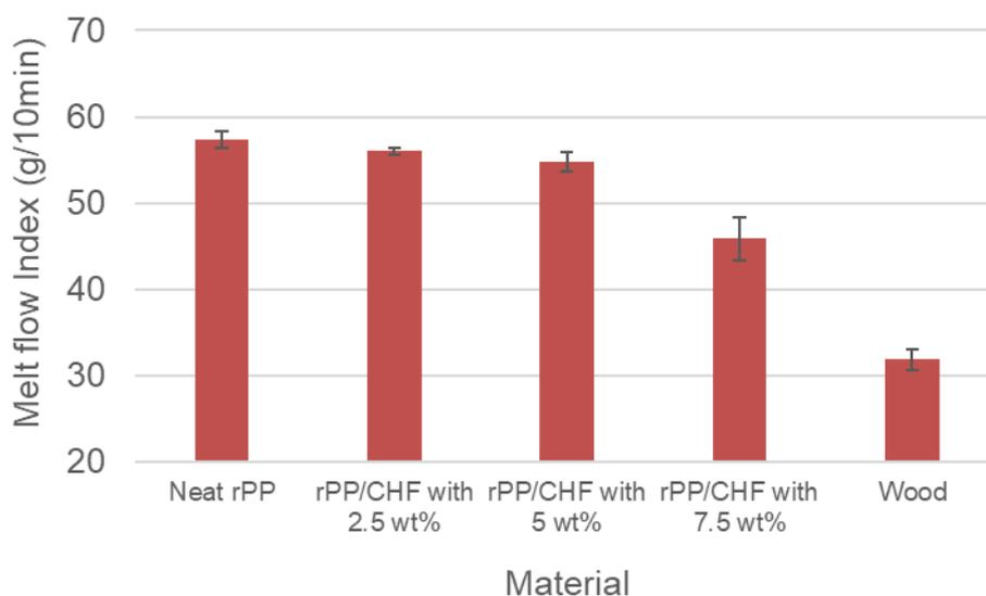
Figure 4.10: Melt flow Index for Different Materials.
