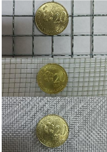
Figure 3.17: Different Sizes of Metal Wire Meshes Compared to 20 cents.
