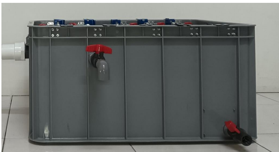
Figure 3.21: Front View of the Grease Separator.
