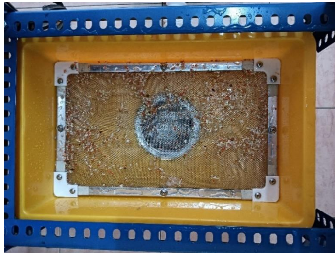
Figure 4.12: Bottom Layer of the Strain Trays After Testing.
