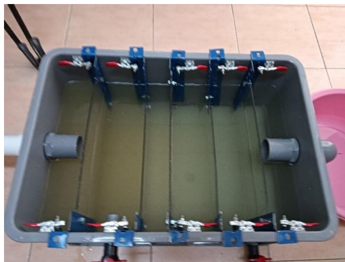
Figure 4.14: Condition of Grease Separator After Testing.
