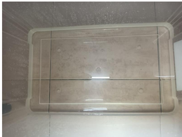
Figure 4.2: Discharged Flow Collected After Mixture 2 Poured into the Grease Separator.
