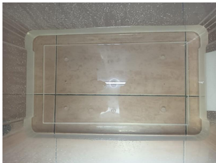
Figure 4.3: Discharged Flow Collected After Mixture 3 Poured into the Grease Separator.
