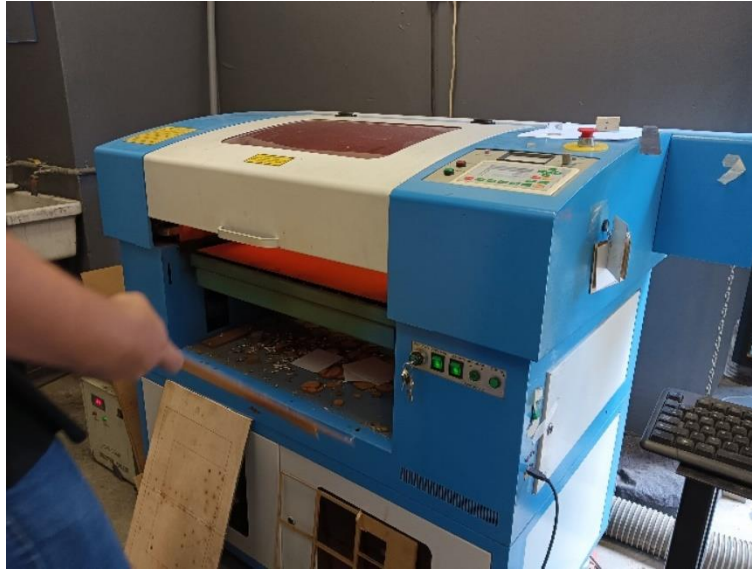
Figure 3.24: Cutting of the Acrylic Sheets through Laser Cutting Machine.
