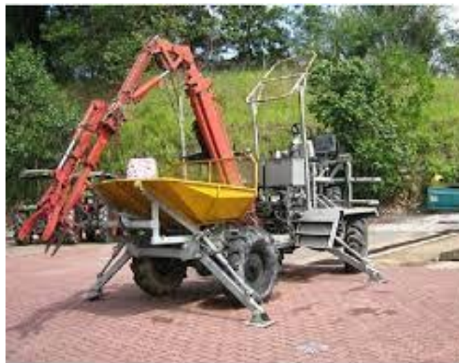
Figure 2.8: Harvester manipulator with robotic arm proposed by Razali et al., (2020)
