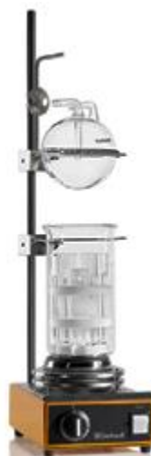
Figure 3.11: Crude Fibre Analyser (Gerhardt Fibrebag-systems 6FBS)
