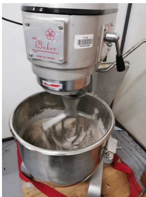
Figure 3.5: Mixing of Dry and Wet Ingredients Using Heavy-duty Mixer
