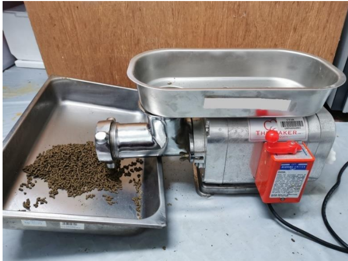
Figure 3.6: Screw-press Extruder Used for Fish Pellets Preparation
