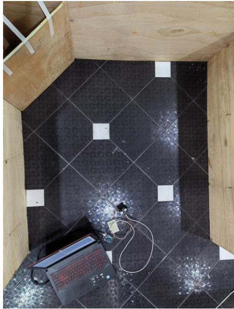
Figure 3.15: Scanning of LiDAR rotate 180-degree with servo motor
