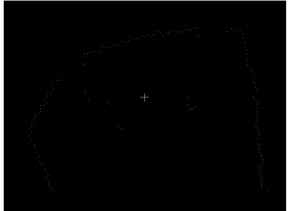
Figure 4.8: Top view of point cloud scanning a single plane with performing averaging of 10 measurements
