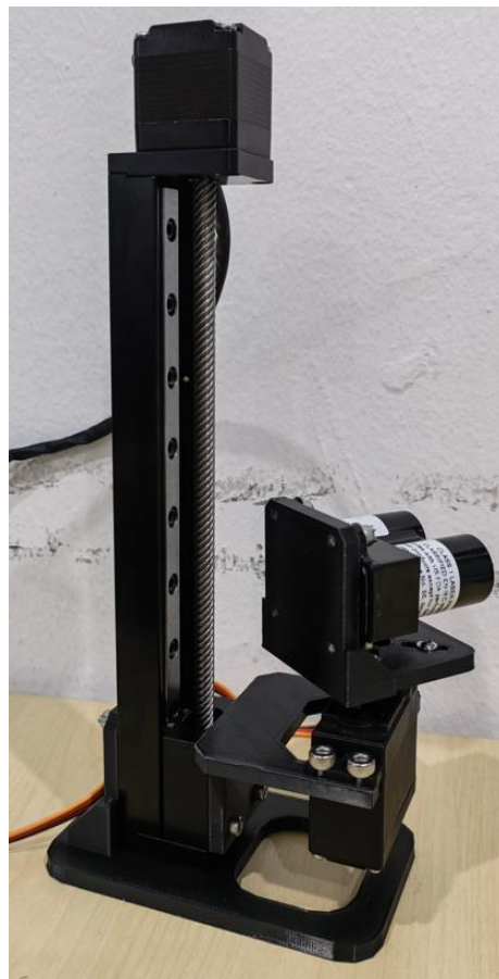
Figure 3.17: Setup of a 3D LiDAR with 3D printed holder.
