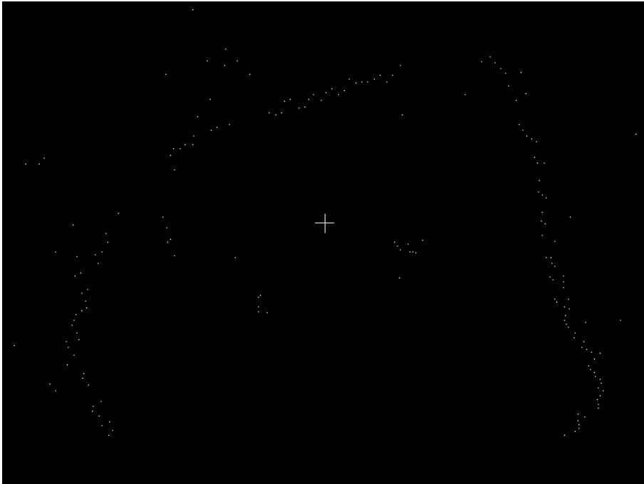
Figure 4.7: Top view of point cloud scanning a single plane without performing averaging
