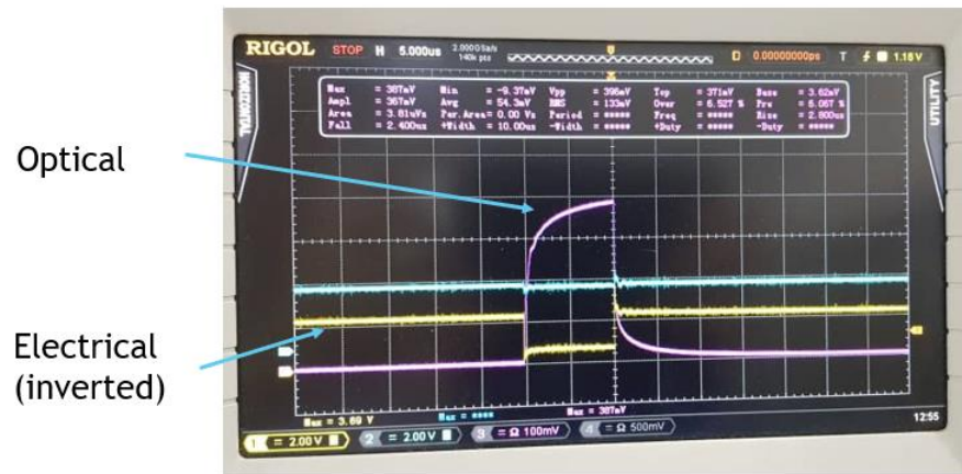
Figure 3.8: Electrical Pulse and Optical Pulse Generated from VCSEL, pulse width 10us, repetition rate 100kHz.
