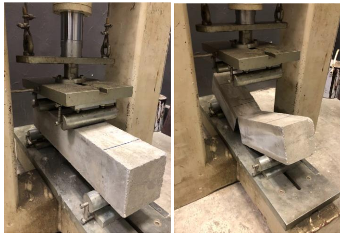
Figure 3.23: Flexural Strength Test (Third Point Loading)
