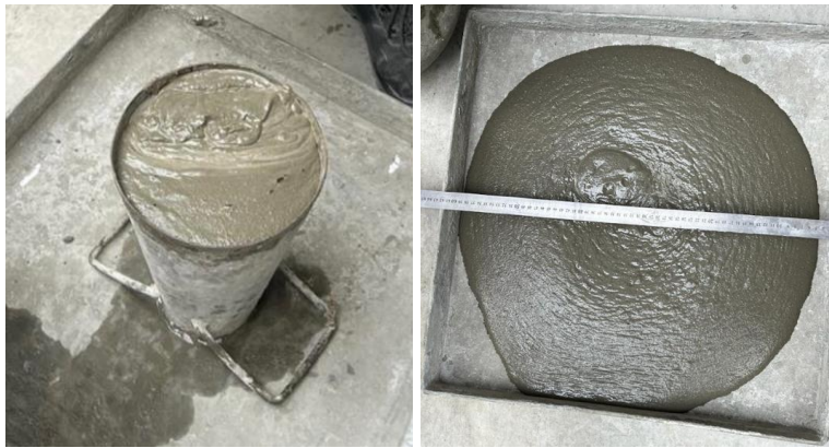
Figure 3.18: Inverted Slump Test
