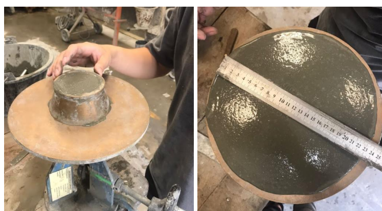
Figure 3.17: Flow Table Test
