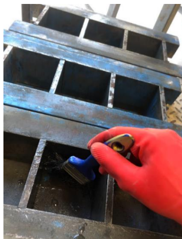
Figure 3.9: Apply Oil Before Casting
