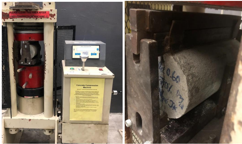
Figure 3.24: Splitting Tensile Test
