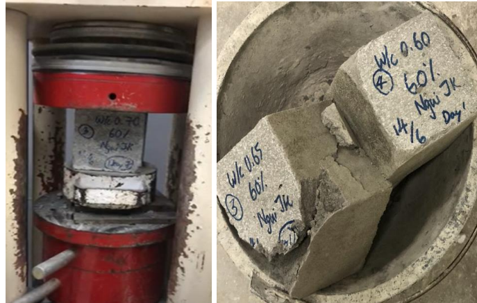
Figure 3.19: Compression test machine.
