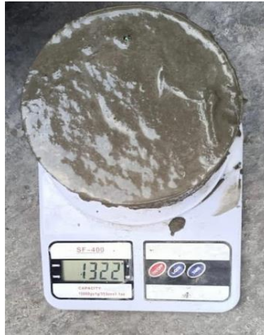
Figure 3.14: Fresh Density Measurement
