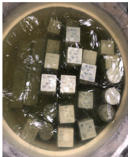
Figure 3.16: Curing Process for the Specimens
