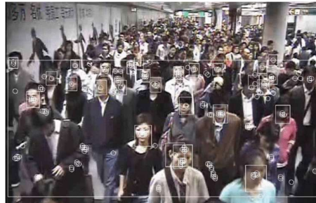
Figure 2.2 : Illustration of face detection. The classifier identified a total of 25 pedestrian from the image. (Keju, Fuqiang and Zhipeng, 2009)
