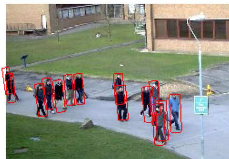
Figure 2.1 : Illustration of fully body detection. There are total of 14 pedestrians in the image. (Ryan, 2010)
