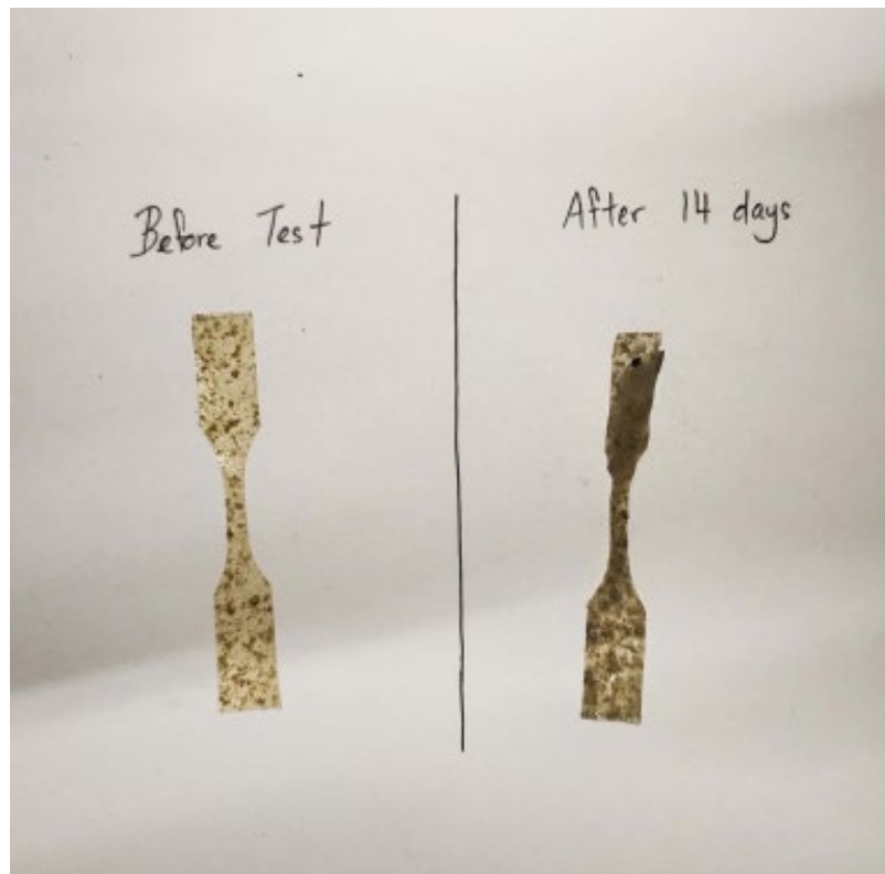
Figure 4.11(a): Biodegradability Test for PVA/CCP Blended Film without lactic acid
