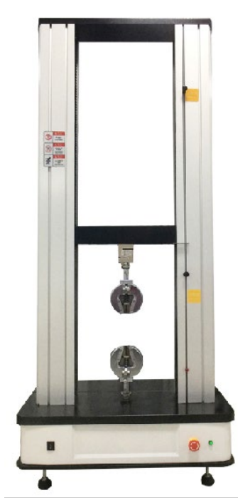
Figure 3.4: Tinius Olsen H10KS-0784 Tensile Testing Machine (Roell, 2022).
