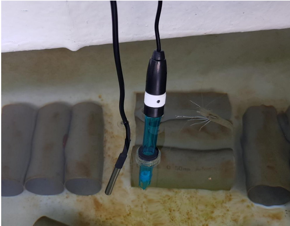
Figure 6.3: DS18B20 and PH4502C Sensor in Water
