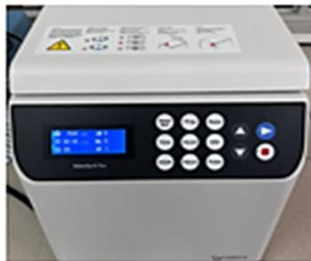
Centrifuge at 7500 rpm for 5 minutes
