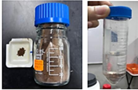
0.02 g of STL was added to 20 mL of CIP solution in 50 mL centrifuge tube
