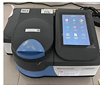
Measurement of absorbance using UV/vis spectrophotometer at 276 nm
