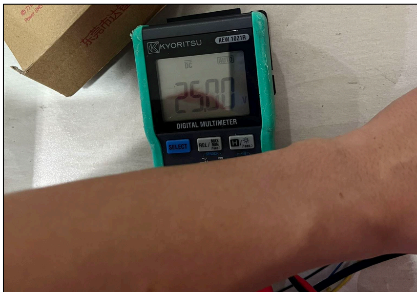
Figure 4.20: The Voltage Measured by the Multi-meter (Trial 3).
