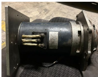
Figure 4.19: Traction Motor AC51-26.26.2 Removed.
