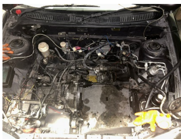
Figure 4.21: Engine Bay after Disassembly of Electric Vehicle Components.
