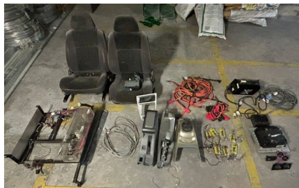
Figure 4.18: Power Electronics and Interior Components Removed from Electric Vehicle.
