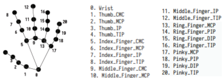
Figure 2.4.1.1: Wrist and upwards as result of normalisation (Suryateja et al., 2022)
