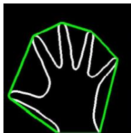
Figure 2.3.1: The convex hull (in green) and the hand contour (in white) (Ismail et al., 2021)
