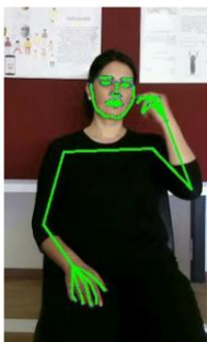
Figure 2.7.1: RGB with whole-body keypoints overlay
