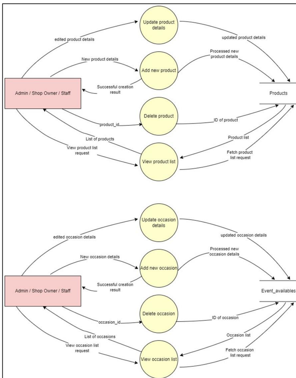
Figure 5.11: Data flow diagram level-1 for Manage Product / Occasion
