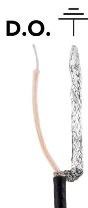
Figure 6.2.12 DO probe central wires and outer wires
