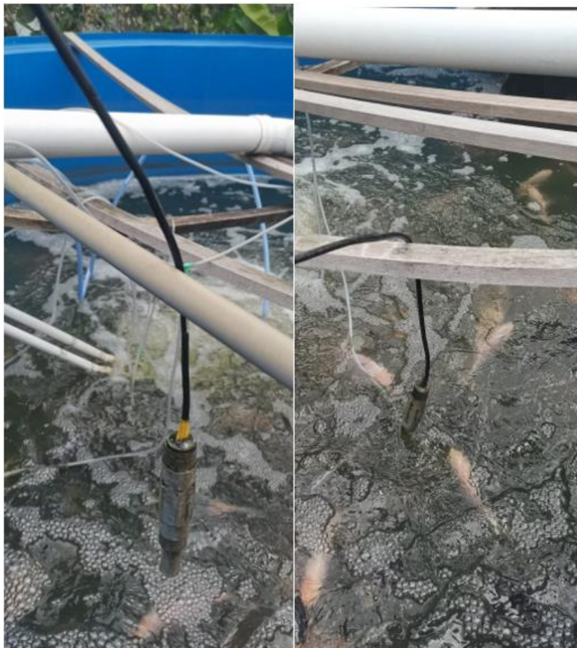
Figure 6.4.3 DO, RTD and PH sensors deployed
