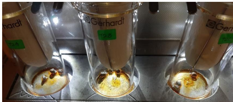
Figure 3.8: End of fat extraction by SOXTHERM®.
