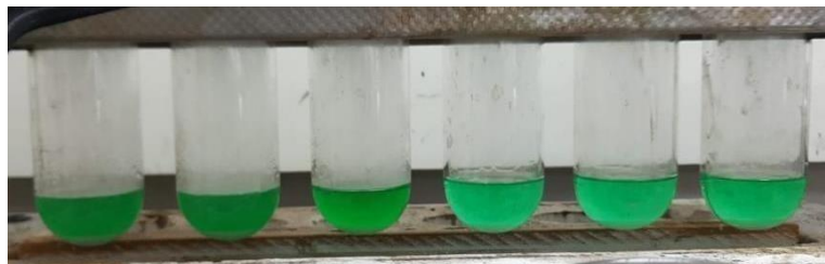
Figure 3.6: End of protein digestion by BUCHI™ Speed Digester.
