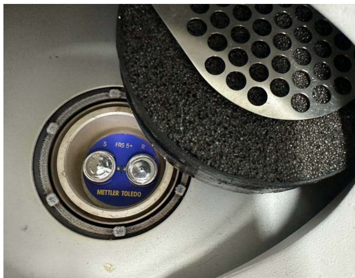
Figure D: DSC furnace with the hermetically sealed aluminum pans loaded in the respective chambers, with “S” representing the sample chamber and “R” representing the reference chamber.
