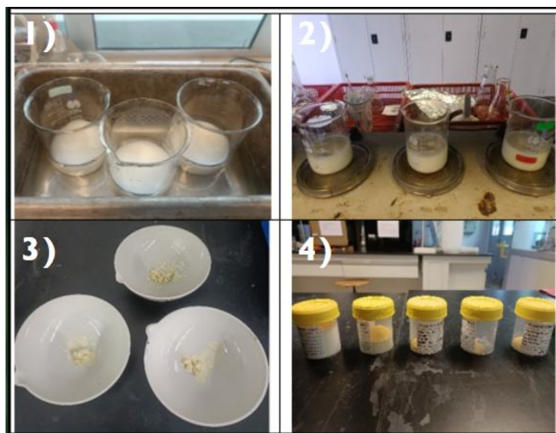
Figure 5.3: Coupling of \text{g-C}_3\text{N}_4 and \text{BiNbO}_4 using simple physical mixing method
