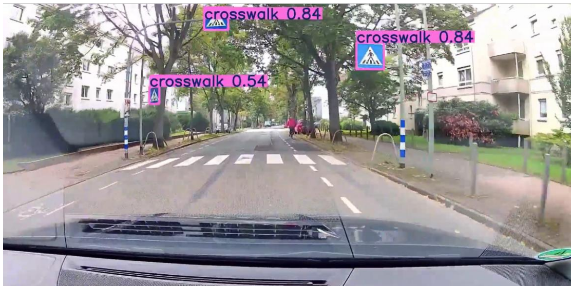
Figure 5.4.3 Sample frame from the output video showing bounding boxes on detected traffic sign
