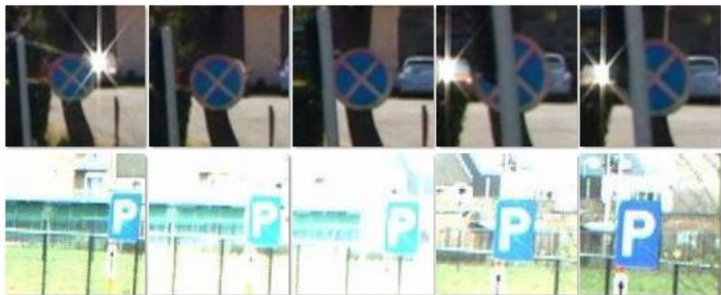
Figure 2.3.2.2 Shows the appearance changes of traffic signs caused by occlusion and illumination
