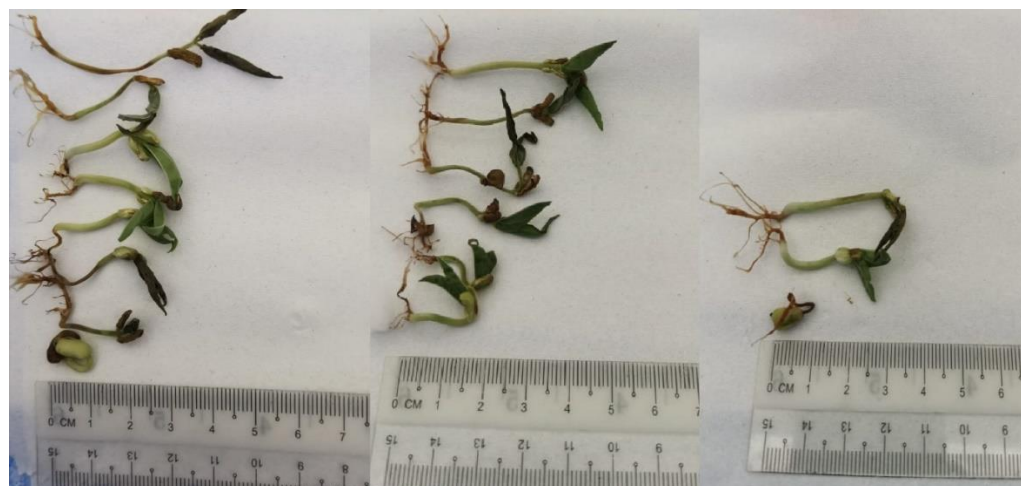
Figure B: Radicle length of Vigna radiata irrigating by (left) distilled water as control; (middle) degraded DMP solution via 10Sr20BWZ photocatalysis and (right) untreated DMP solution.
