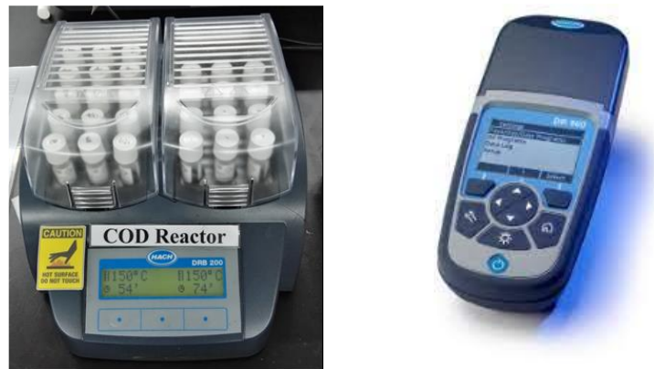
Figure 3.5: COD Reactor (DRB 200) and Colorimeter (DR 900)
