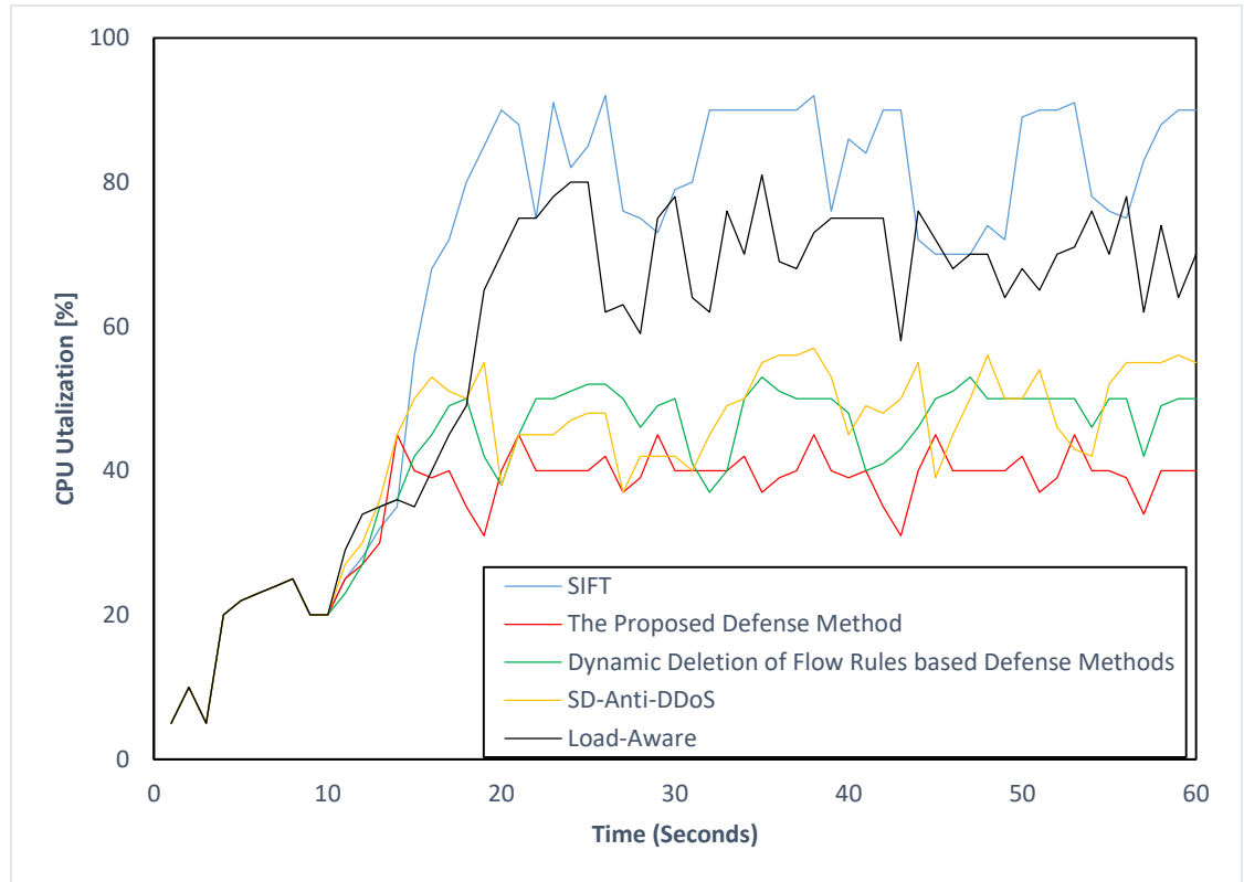
Figure 5.7: Comparison of the proposed defense method with existing methods in terms of CPU utilization.
