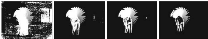
Figure 2.17: Effects of unsuitable threshold value. An inappropriate threshold value will cause noise in the frame difference, which would cause noise in the final MHI. The threshold value is set at 30, 50, 74, and 150 from left to right, respectively. A noisy background is noted with a threshold value of 30, yet some motion information is missing with a higher value [71].
