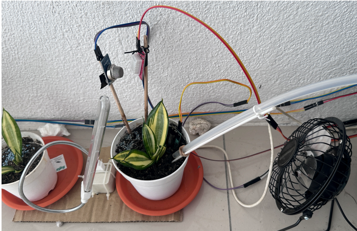
Figure 17 DHT22 Sensor, MQ-135 Sensor, Water pipe, Fan and Full Spectrum LED set up on the plant
