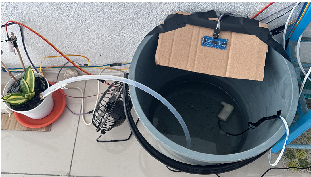
Figure 16 Water pump (in the water) and Ultrasonic Sensor to detect water level
