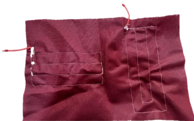
Figure 3.3.4: Prototype of a Single Sensor Node with 0.2 mm Stainless Steel
