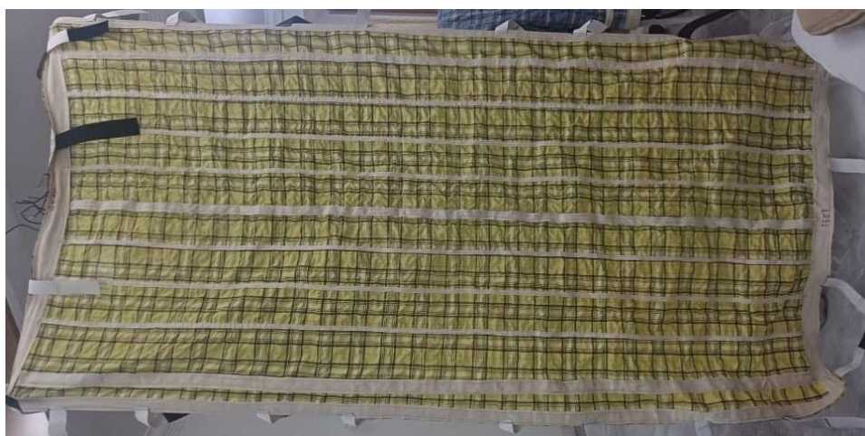
Figure 3.3.5: VT8 Prototype Sensor Layer: Eight vertical sensor lines.
