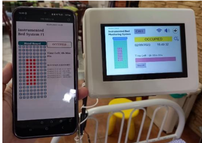
Figure 3.7.3: Device user interface: Web-based (left), Touchscreen (Right)
