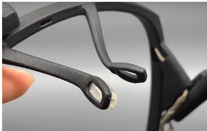
Figure 2.5: Pupil Core Headset with Nose Support Equipped with a Silicon Nose Pad (Pupil Labs, 2023e).
