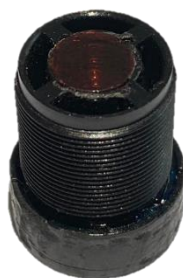
Figure 3.8: Replacement of IR Filter with Exposed Film.
