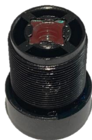
Figure 3.7: IR filter in the Lens of Camera Module.
