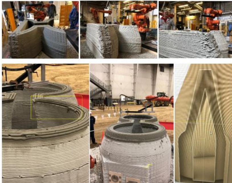
Figure 1: (Above) Experimental exploration of diverse edge configurations and material deformation at the edges in the process of robotic 3D printing. (Below) Bead failure on the interior side of a tapering cone (indicated by a dotted yellow line). (Lower right) Cross-sectional representation of the module's geometry at the connector, highlighting fillet edges (Muthumanickam et al., n.d.).
